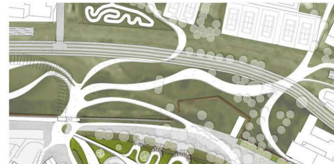
Covering the railway tunnel by a layer of soil and greenery. The vehicular road became one avenue with sidewalks, bicycle lanes, vehicular lanes. Each lane is separated from the other by greenery. Crossing points, zebra lines, lights, bumps are added to reduce car speed and assure safe pedestrian circulation and crossing.
