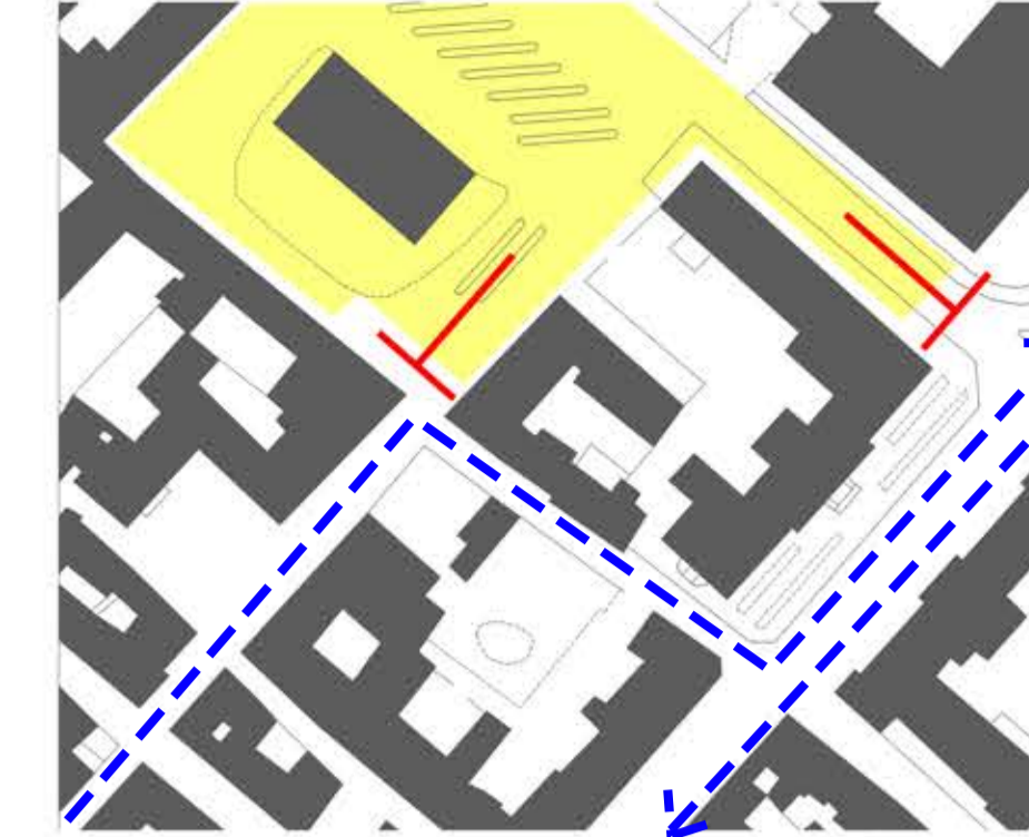
Car dominance in the Piazza in completely substituted by pedestrian dominance. Vehicular access to the Piazza are prohibited. Via Bacciochi is blocked for car circulation. Concerning Via cittadella, cars are diverted to Via Risorgimento through Via Gregorio X.
