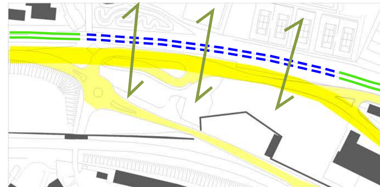
Moving the railway underground for a length of 270meters. Simplifying the vehicular road network by making it one linear road, which make crossing of people easier.
