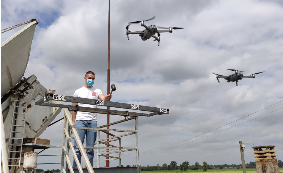
Figure 4.9: Setup of the second test. Drones are positioned such that each one is unable to capture the whole structure.
