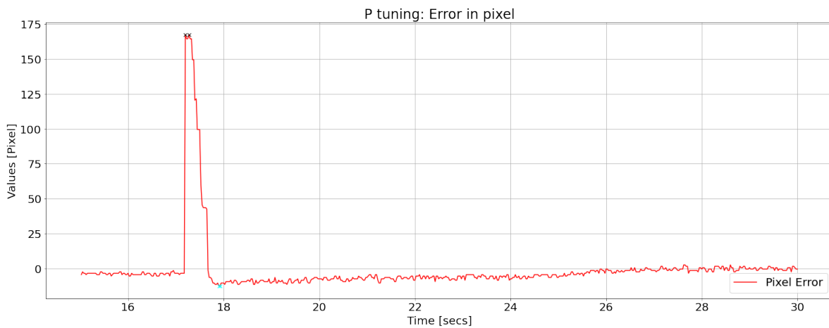
Figure 5.9: Error in the image space along x direction ( K_{Px} = 0.5, K_{Py} = 0 ).
