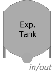
Figure 1.3: The expansion vessel in the DHN4Control Modelica library.
