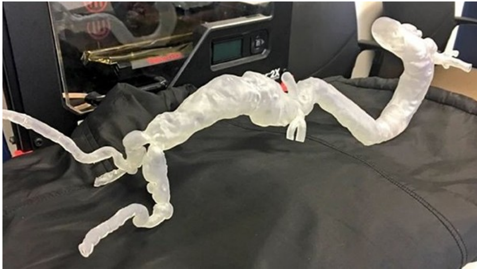
Figure 2.10: Example of a thin-walled silicone vascular phantom reproducing a patient-specific pathological arterial geometry [18]. The phantom was developed for experimental evaluation and training in catheter-based endovascular procedures.
