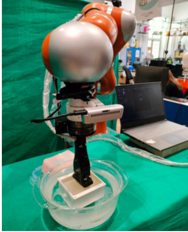
Figure 3.13: In-vitro US acquisition setup with probe pose tracking via robotic arm.
