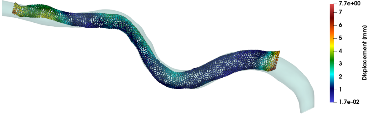
Figure 4.6: Estimated displacement field introduced by the non-rigid registration exemplified for the Artery phantom. Points of the intraoperative reconstruction are colored according to displacement magnitude (in mm), illustrating the spatial distribution of the applied correction.
