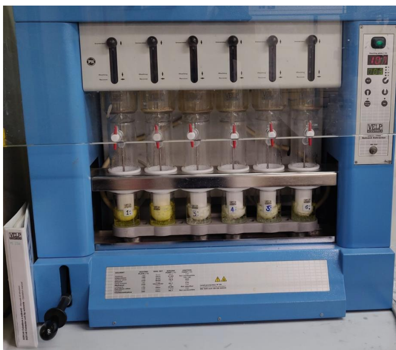
Figure 3. 3 - Soxhlet solvent extractor VELP SER 148.
