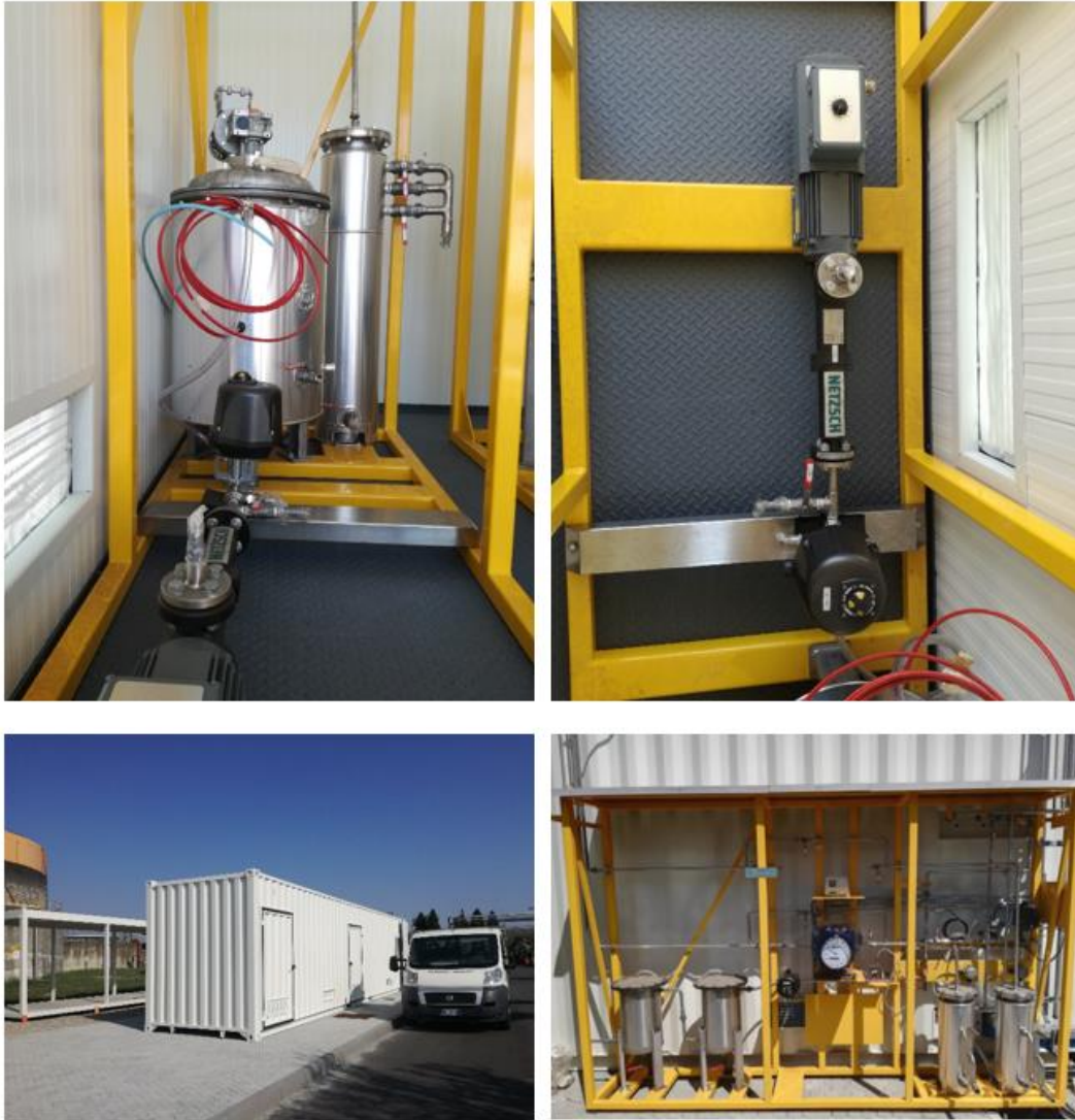
Figure 3. 2 - Pictures of the anaerobic digester, the pump, the internal and external hydraulic seals and the container before the start-up.
