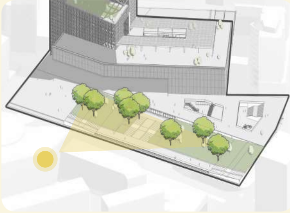
Natural solar protection - plaza
