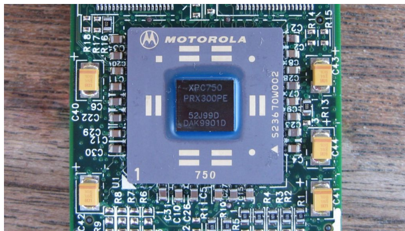
Figure 8: Processor used for Perseverance, taken from a Mac dated 1997
