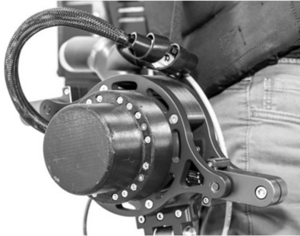
Figure 11 Picture of the parallel-elastic actuator on the Robo-Mate active trunk. The spring is implemented with a bungee cord and acts in parallel to a gear motor, hidden by the black cover in this picture (Sharit, 2020).
