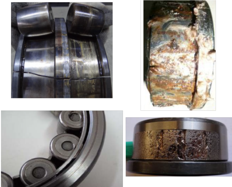
Figure 6.5: Fault bearings due to lack of lubrication (top-left), contamination (top-right), misalignment (bottom-left) and fatigue related wear (bottom-right). Pictures from [83]
