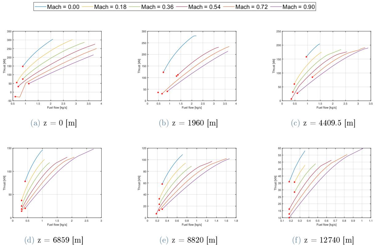
Figure 4.23: Thrust vs Fuel flow plots of GENx-1B64.
