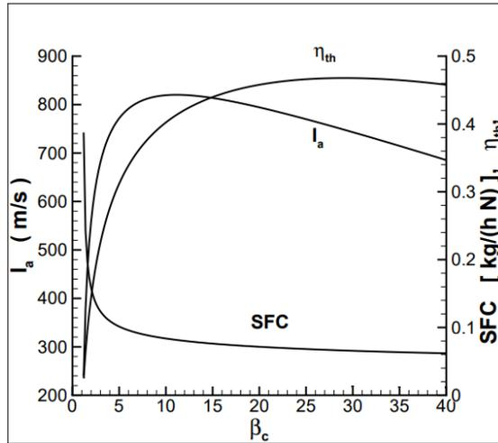
Figure 2.9: Effect of  $\beta_c$  on  $SFC$ ,  $\eta_{th}$  and  $I_a$ . It is possible to observe that  $SFC$  and  $\eta_{th}$  are linked each other, instead  $I_a$  has a different trend [11].
