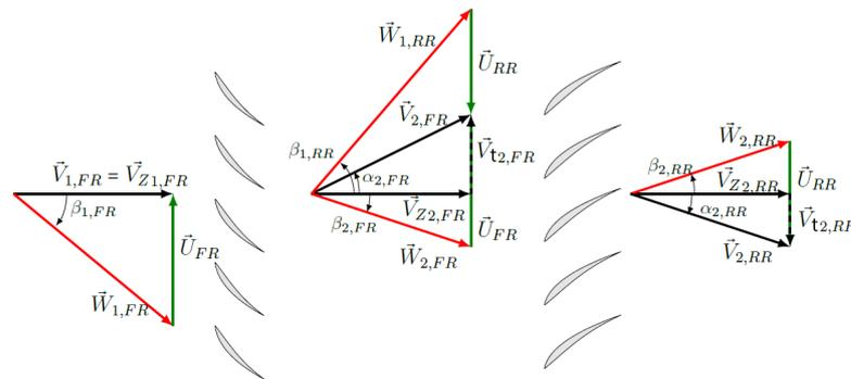
Figure 2.8: Counter-rotating fan: counter Rotor-Rotor stage [32]
