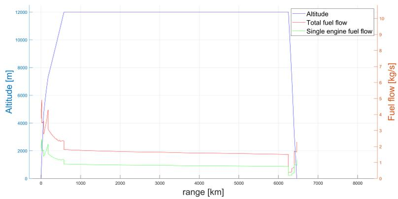
Figure 7.40: Reference long mission: Altitude and Fuel flow vs range.
