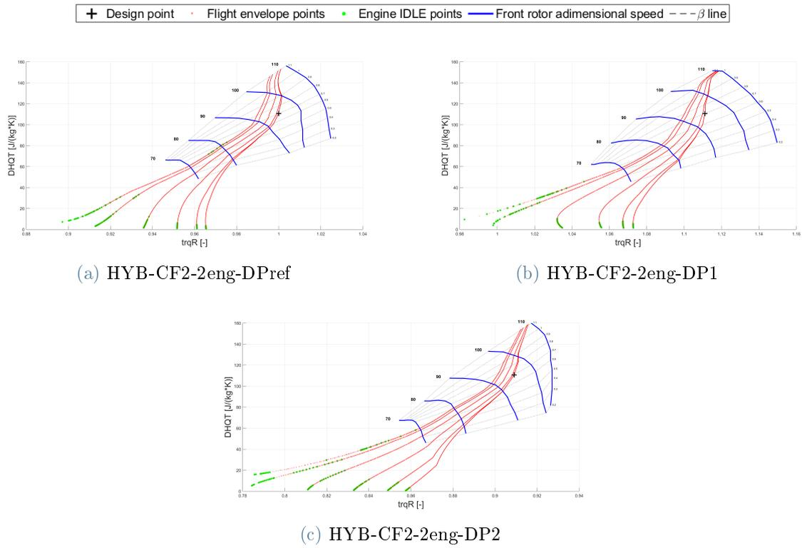
Figure 5.12: CR fan engines HYB-CF2-2eng: torque ratio maps.
