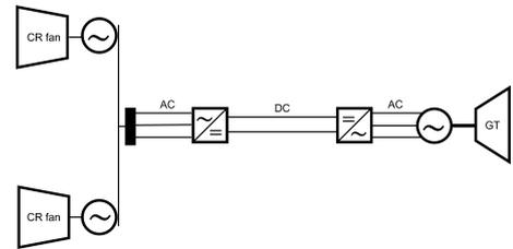
(b) Tu-el pc with 2 electric CR fan engines.
