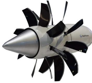
Figure 2.7: Safran open rotor model, 2017
