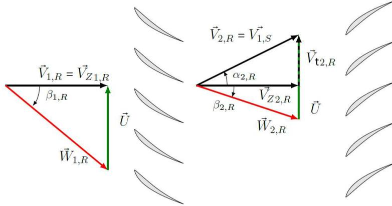
Figure 2.6: Axial compressor: Rotor-Stator stage [32].
