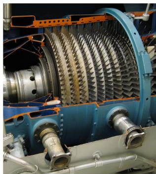
Figure 2.2: View of an axial HP compressor in a Pratt & Whitney TF30 turbofan engine.
