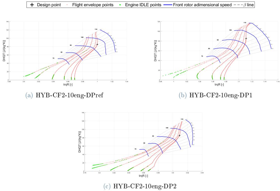
Figure 5.15: CR fan engines HYB-CF2-10eng: torque ratio maps.
