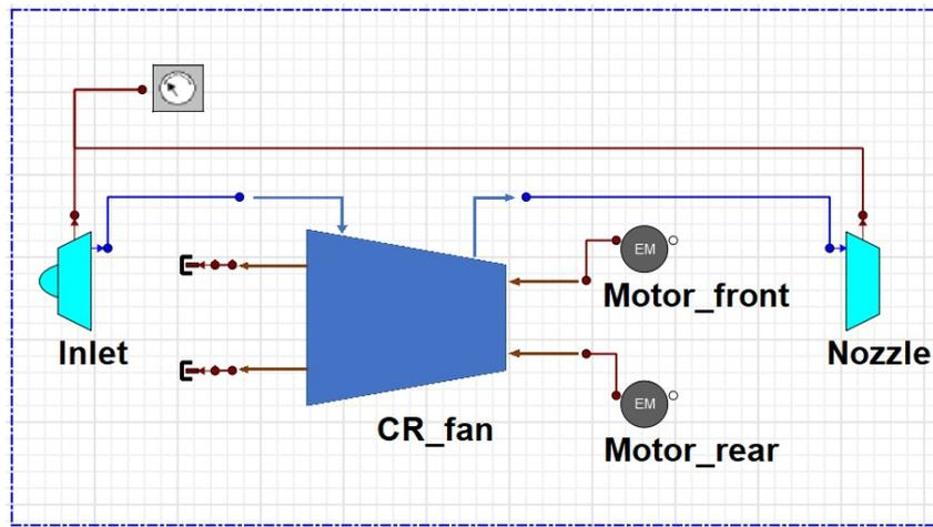
Figure 5.2: HYB-CF1 schematic.
