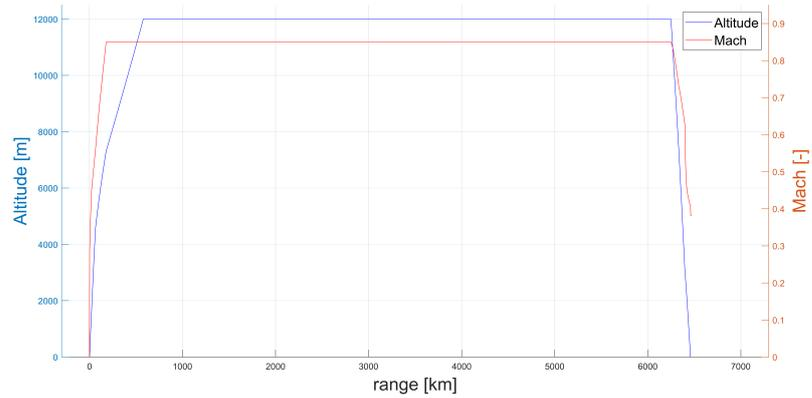
Figure 7.42: Reference long mission: Altitude and Mach vs range.
