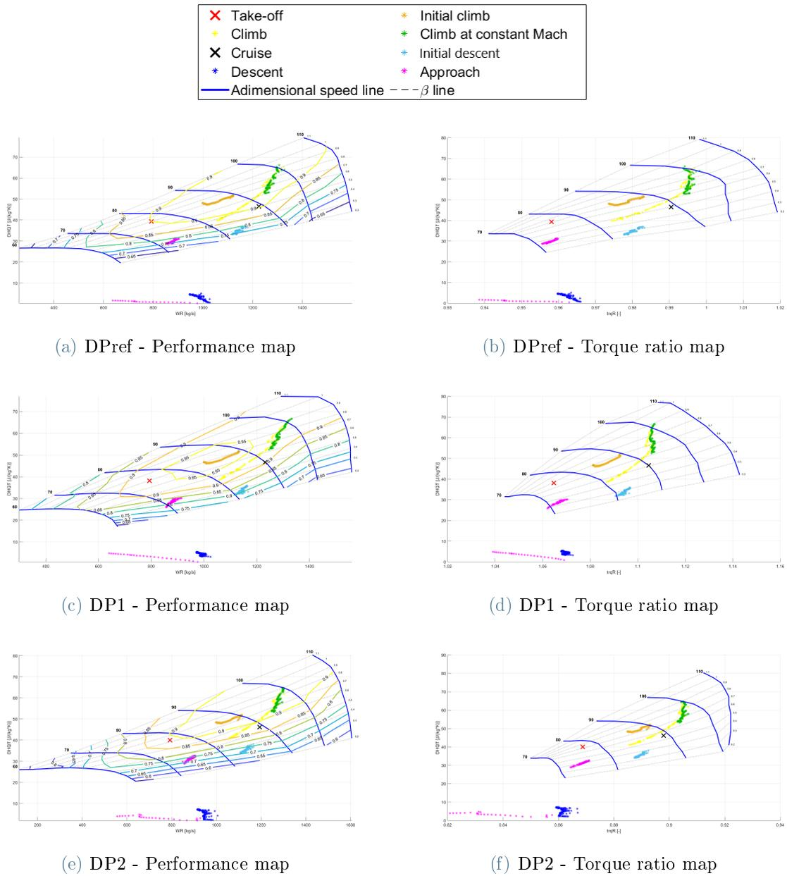
Figure 7.17: CR fan engines HYB-CF1-2eng in a short range mission, CASE 1: CR fan performance points during flight.
