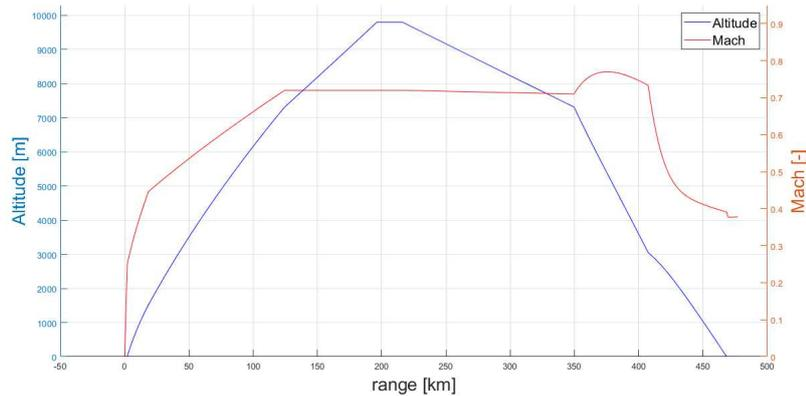
Figure 7.12: Reference short mission: Altitude and Mach vs range.
