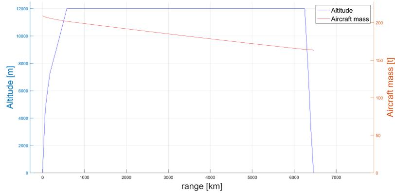
Figure 7.41: Reference long mission: Altitude and Aircraft mass vs range.
