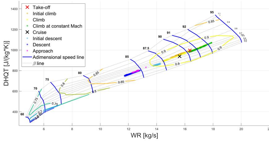
Figure 7.8: Reference short mission: CFM56-7B24 HP compressor performance points during flight.
