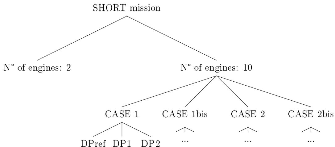
Figure 7.20: Tree diagram that describes the sensitivity analysis procedure in the case of short mission range in 10 engines configuration.
