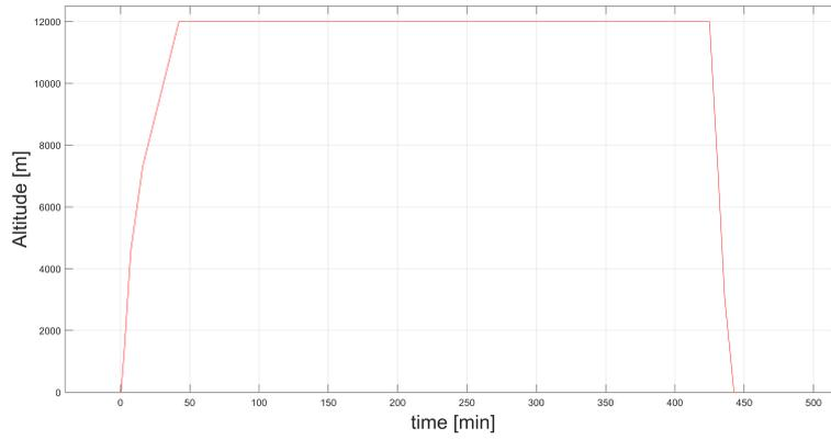
Figure 7.38: Reference long mission: Altitude vs time of flight.
