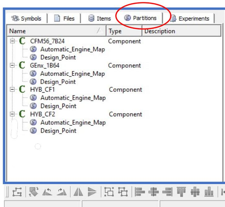
Figure 3.2: For each schematic built (CFM56-7B24, GENx-1B64, HYB-CF1 and HYB-CF2), two partitions has been generated: "Automatic\_Engine\_Map" and "Design\_Point". The first one is referred to the off-design analysis, the second one is referred to the design analysis (i.e. design model partition).
