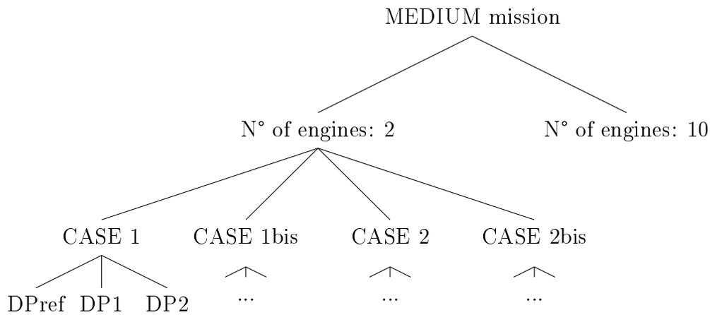
Figure 7.31: Tree diagram that describes the sensitivity analysis procedure in the case of medium mission range in 2 engines configuration.
