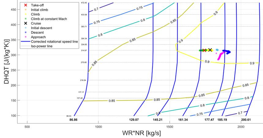
Figure 7.10: Reference short mission: CFM56-7B24 LP turbine performance points during flight.
