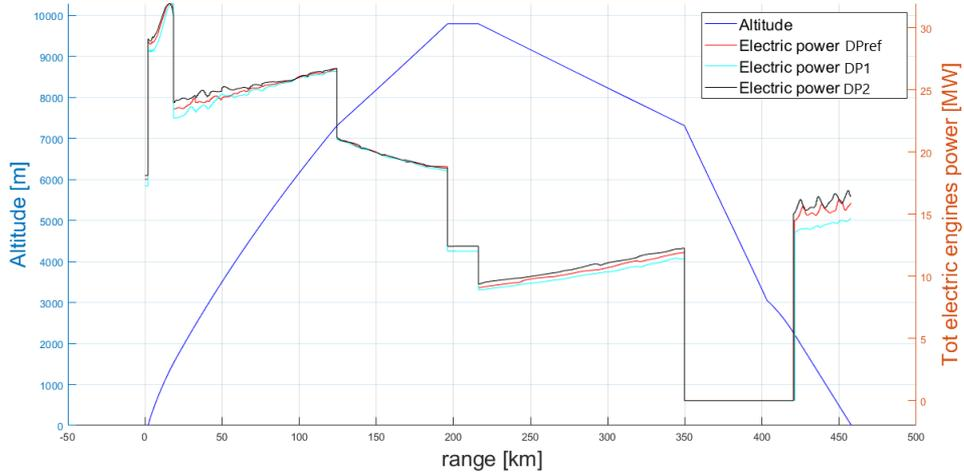
Figure 7.18: Short range mission CASE 1 in 2 engines configuration: Altitude and Tot electric motors power vs Range, results comparison between the CR fan engines HYB-CF1-2eng-DPref, HYB-CF1-2eng-DP1 and HYB-CF1-2eng-DP2.
