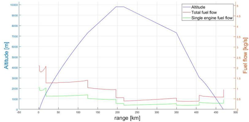
Figure 7.14: Reference short mission: Altitude and Fuel flow vs range.
