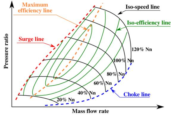
Figure 2.3: Typical operating curve for an axial compressor [40].
