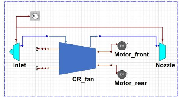
Figure 5: Electric CR fan schematic.
