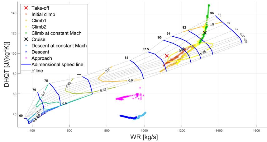
Figure 7.33: Reference long mission: GEnx-1B64 fan performance points during flight.
