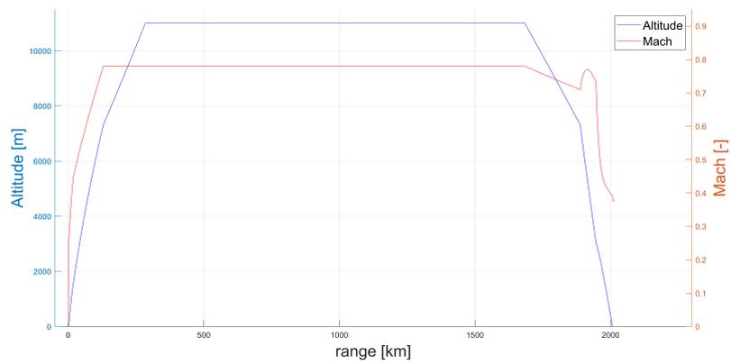
Figure 7.30: Reference medium mission: Altitude and Mach vs range.
