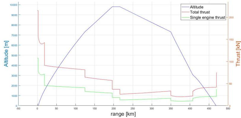
Figure 7.13: Reference short mission: Altitude and Thrust vs range.
