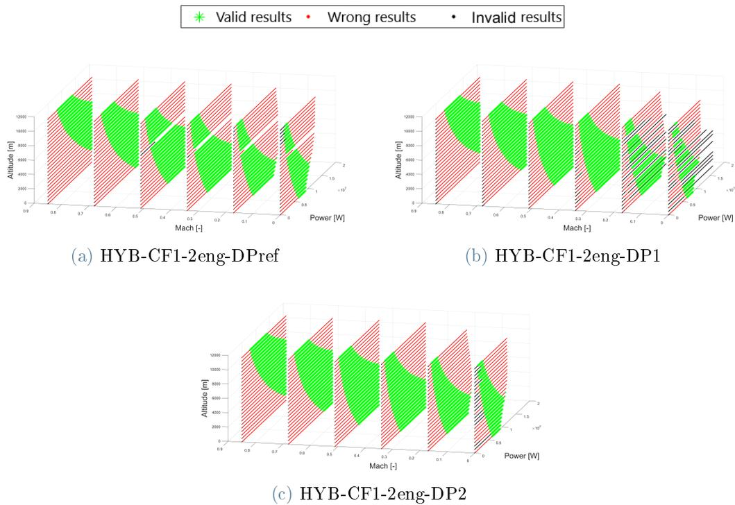
Figure 5.5: HYB-CF1-2eng engine maps with no extended results.
