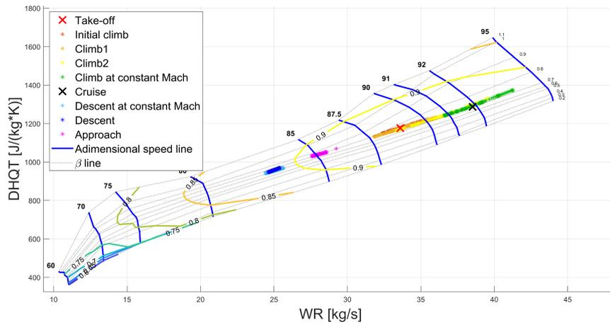
Figure 7.35: Reference long mission: GENx-1B64 HP compressor performance points during flight.
