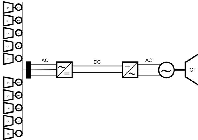
Figure 7.4: Tu-el pc with 10 electric CR fan engines. This configuration is used in CASE 2 and CASE 2bis. For each one of these two CASEs the electric CR fan engines can be part of the HYB-CF1-10eng or HYB-CF2-10eng series. The total number of electric engines is 20.
