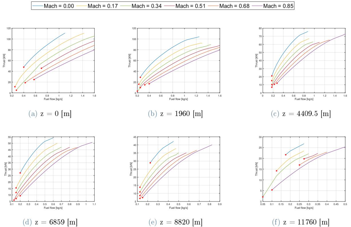
Figure 4.12: Thrust vs Fuel flow plots of CFM56-7B24.
