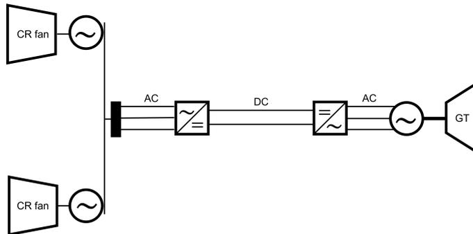
Figure 7.3: Tu-el pc with 2 electric CR fan engines. This configuration is used in CASE 2 and CASE 2bis. For each one of these two CASEs the electric CR fan engines can be part of the HYB-CF1-2eng or HYB-CF2-2eng series. The total number of electric engines is 4.
