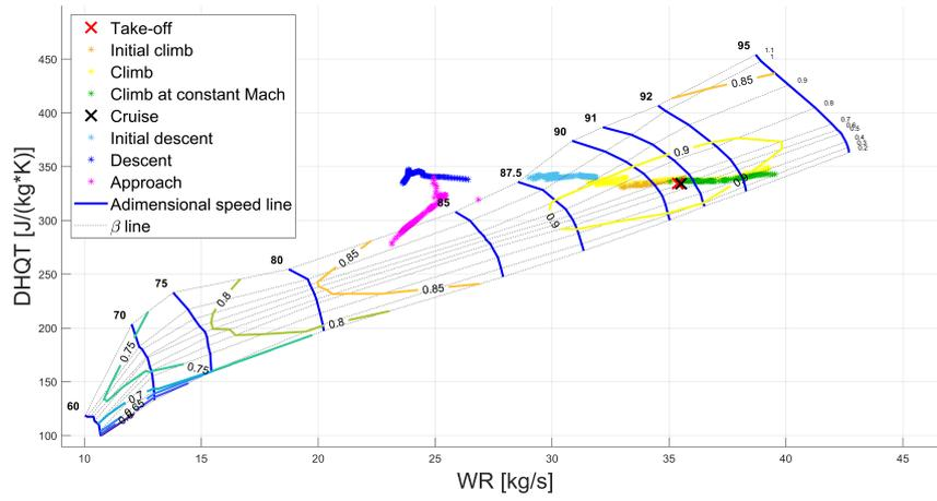
Figure 7.22: Reference medium mission: CFM56-7B24 LP compressor performance points during flight.
