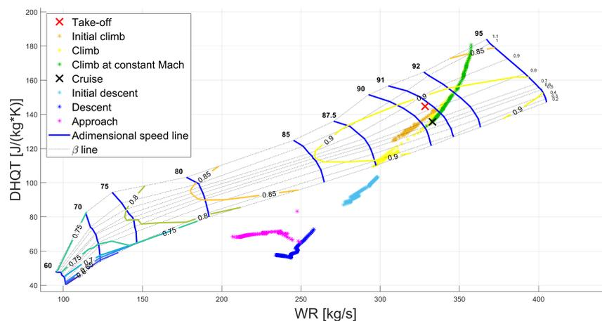
Figure 7.21: Reference medium mission: CFM56-7B24 fan performance points during flight.
