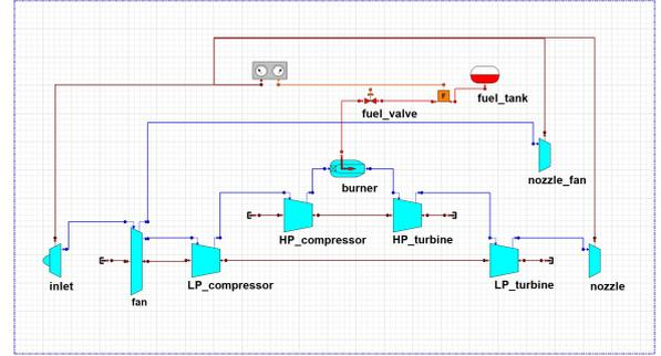
Figure 4: Turbofan schematic.
