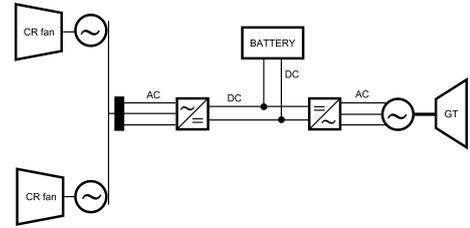
(a) Hy-el se with 2 electric CR fan engines.
