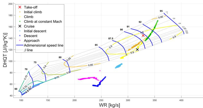
Figure 7.6: Reference short mission: CFM56-7B24 fan performance points during flight.
