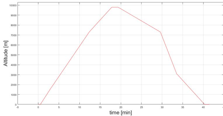
Figure 7.11: Reference short mission: Altitude vs time of flight.
