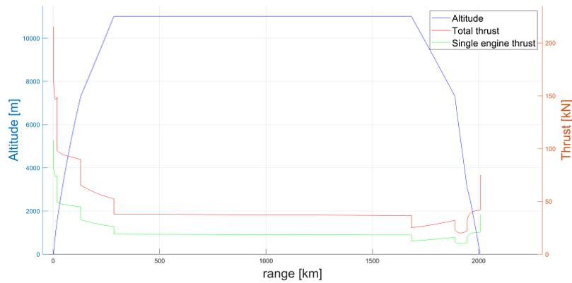
Figure 7.27: Reference medium mission: Altitude and Thrust vs range.
