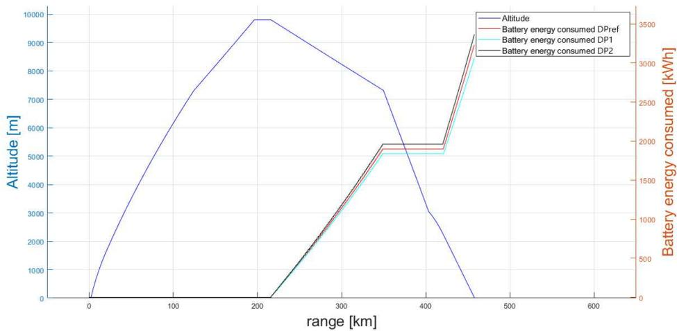
Figure 7.19: Short range mission CASE 1 in 2 engines configuration: Altitude and Battery energy consumed vs Range, results comparison between the CR fan engines HYB-CF1-2eng-DPref, HYB-CF1-2eng-DP1 and HYB-CF1-2eng-DP2.
