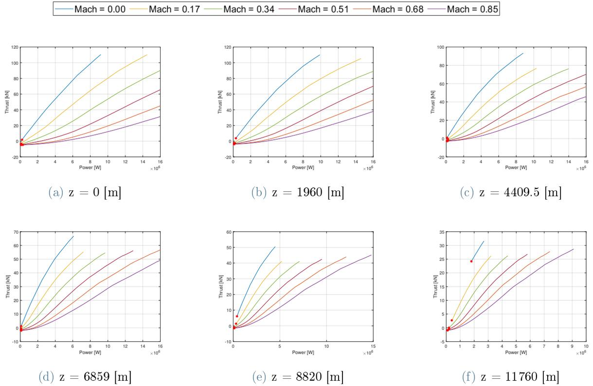
Figure 5.7: HYB-CF1-2eng-DPref: Thrust vs Power plots.
