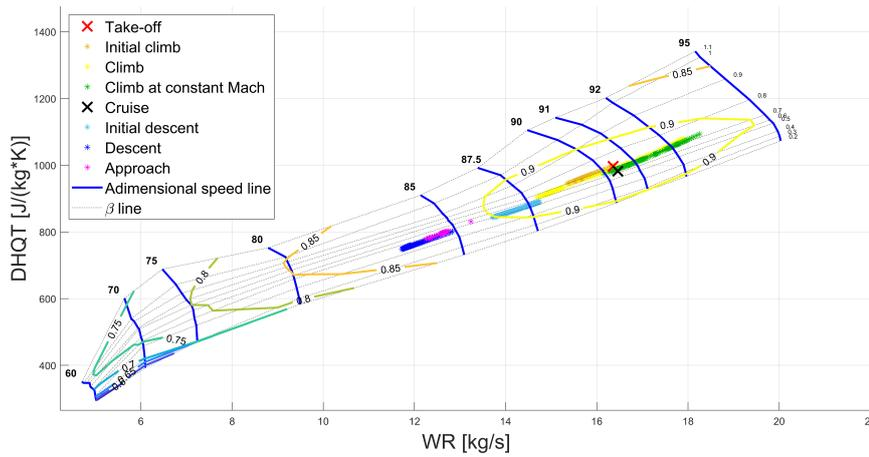
Figure 7.23: Reference medium mission: CFM56-7B24 HP compressor performance points during flight.
