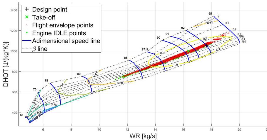
Figure 4.5: CFM56-7B24 HP compressor performance map.
