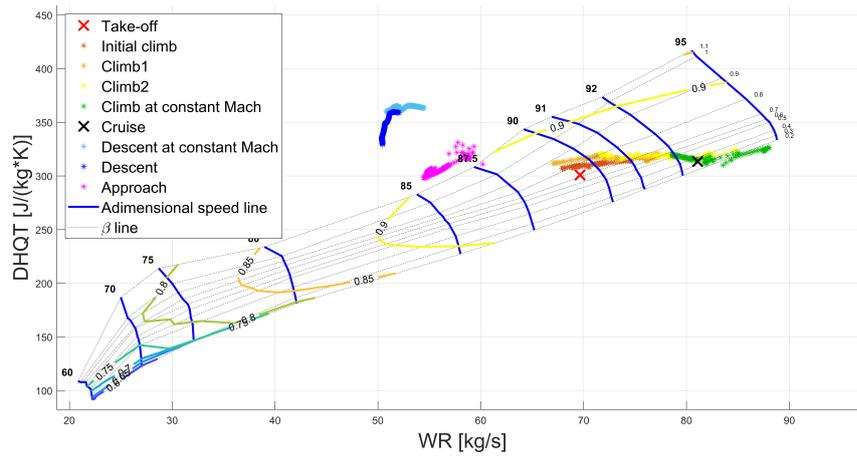
Figure 7.34: Reference long mission: GEnx-1B64 LP compressor performance points during flight.
