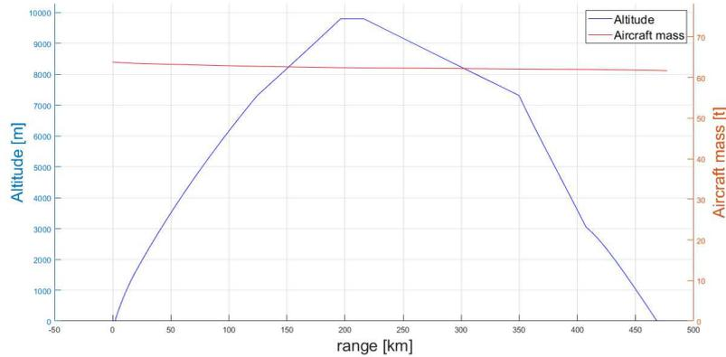
Figure 7.15: Reference short mission: Altitude and Aircraft mass vs range.
