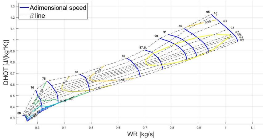
Figure 3.5: Non-scaled fan and compressor performance map.
