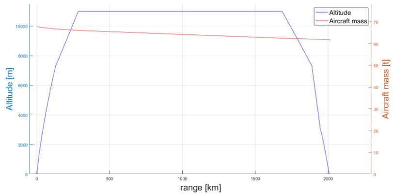
Figure 7.29: Reference medium mission: Altitude and Aircraft mass vs range.
