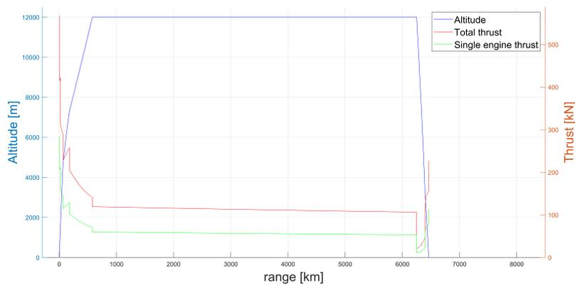
Figure 7.39: Reference long mission: Altitude and Thrust vs range.
