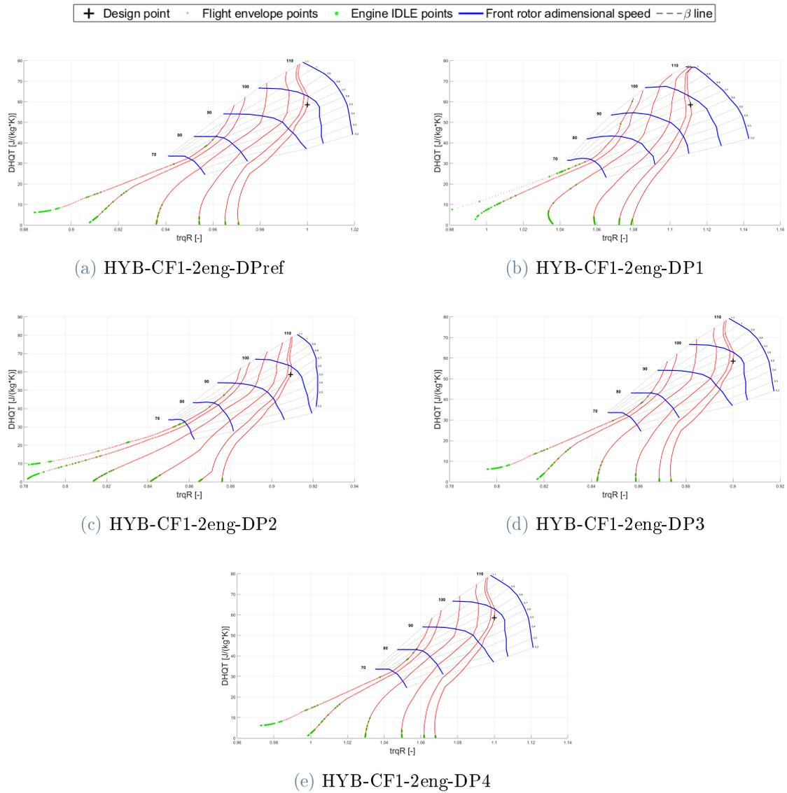
Figure 5.3: CR fan engines HYB-CF1-2eng: torque ratio maps.
