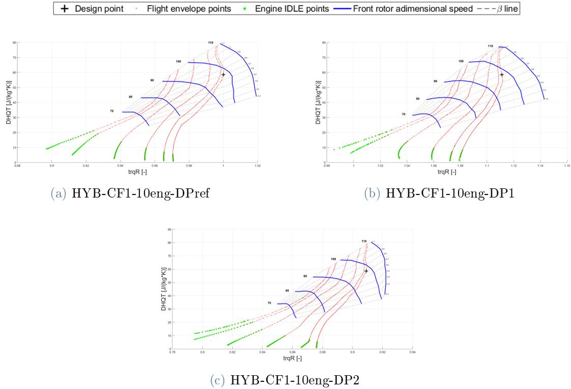
Figure 5.8: CR fan engines HYB-CF1-10eng: torque ratio maps.
