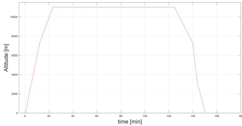
Figure 7.26: Reference medium mission: Altitude vs time of flight.
