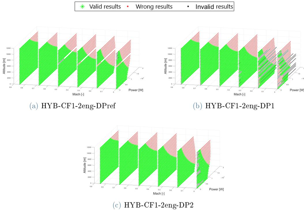
Figure 5.6: HYB-CF1-2eng engine maps with extended results.
