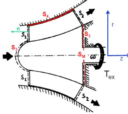
Figure 2.4: Control volume used to demonstrate the Euler work [12].
