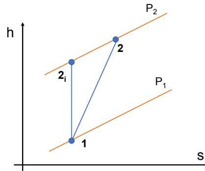
Figure 3.6: T-s diagram: Compressor isentropic efficiency.
