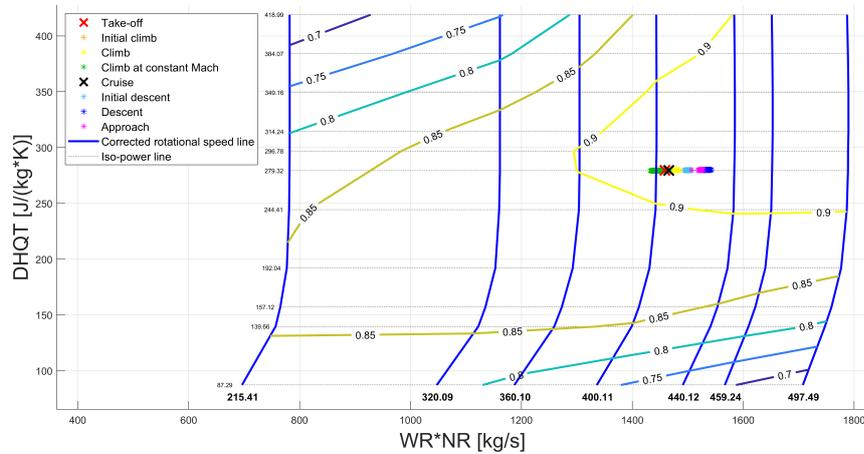
Figure 7.24: Reference medium mission: CFM56-7B24 HP turbine performance points during flight.
