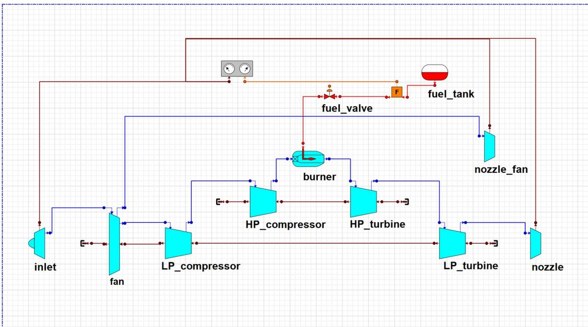
Figure 4.2: CFM56-7B24 schematic.
