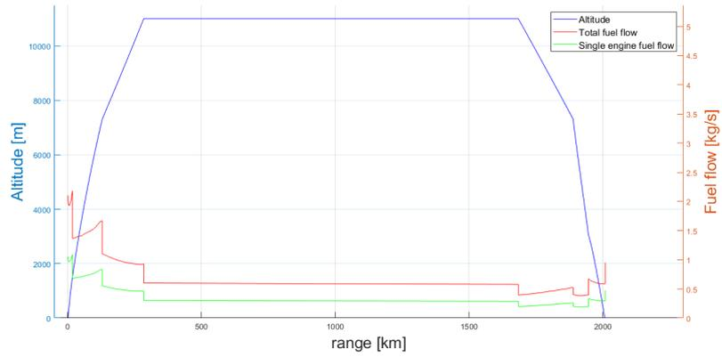
Figure 7.28: Reference medium mission: Altitude and Fuel flow vs range.
