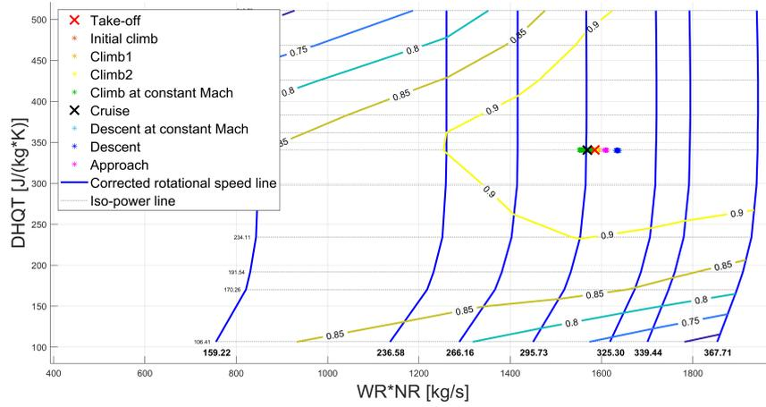
Figure 7.36: Reference long mission: GENx-1B64 HP turbine performance points during flight.
