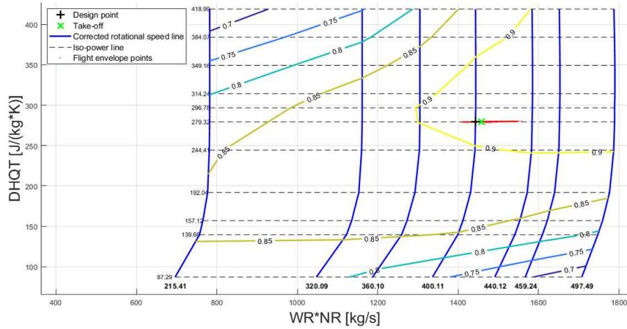
Figure 4.8: CFM56-7B24 HP turbine performance map.
