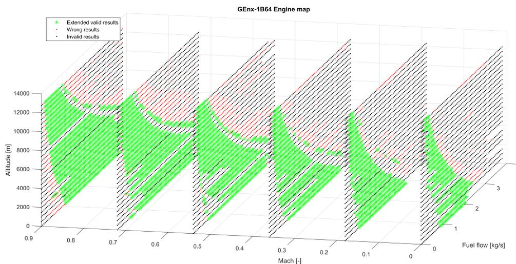
Figure 4.22: GEnx-1B64: Engine map with extended results.
