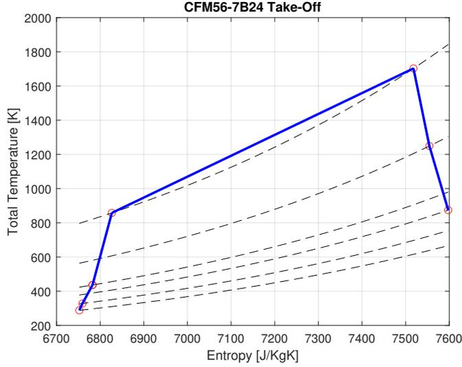
Figure 4.13: CFM56-7B24 thermodynamic cycle in take-off condition.
