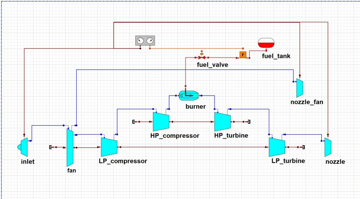
Figure 4.15: GEEnx-1B64 schematic.
