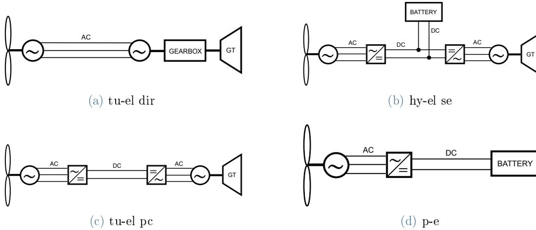
Figure 2.10: Hybrid propulsion systems.
