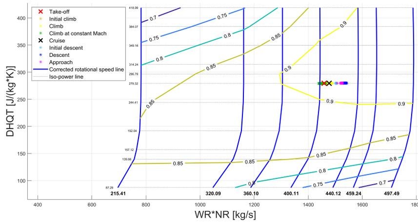
Figure 7.9: Reference short mission: CFM56-7B24 HP turbine performance points during flight.
