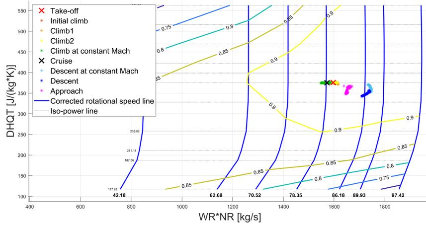
Figure 7.37: Reference long mission: GENx-1B64 LP turbine performance points during flight.
