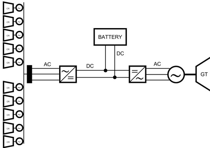
Figure 7.2: Hy-el se with 10 electric CR fan engines. This configuration is used in CASE 1 and CASE 1bis. For each one of these two CASEs the electric CR fan engines can be part of the HYB-CF1-10eng or HYB-CF2-10eng series. The total number of electric engines is 20.
