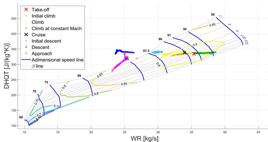
Figure 7.7: Reference short mission: CFM56-7B24 LP compressor performance points during flight.
