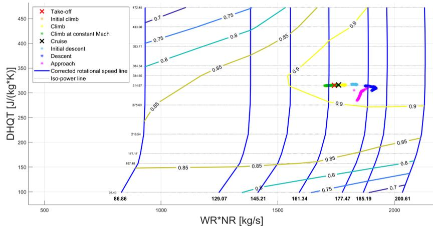
Figure 7.25: Reference medium mission: CFM56-7B24 LP turbine performance points during flight.
