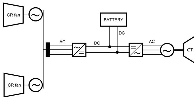
Figure 7.1: Hy-el se with 2 electric CR fan engines. This configuration is used in CASE 1 and CASE 1bis. For each one of these two CASEs the electric CR fan engines can be part of the HYB-CF1-2eng or HYB-CF2-2eng series. Remember that each CR fan engine is propelled by two electric engines, one for each shaft. Therefore, for example, in this case the total number of electric engines is 4.
