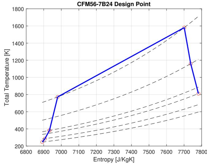
Figure 4.3: CFM56-7B24 thermodynamic cycle in design point (i.e. cruise) condition.
