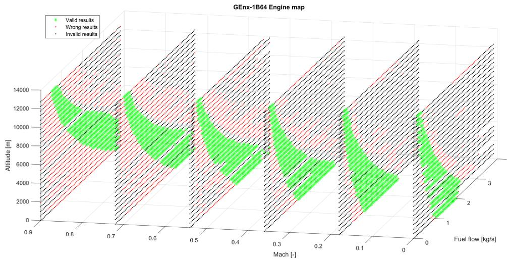
Figure 4.21: GEnx-1B64: Engine map with no extended results.
