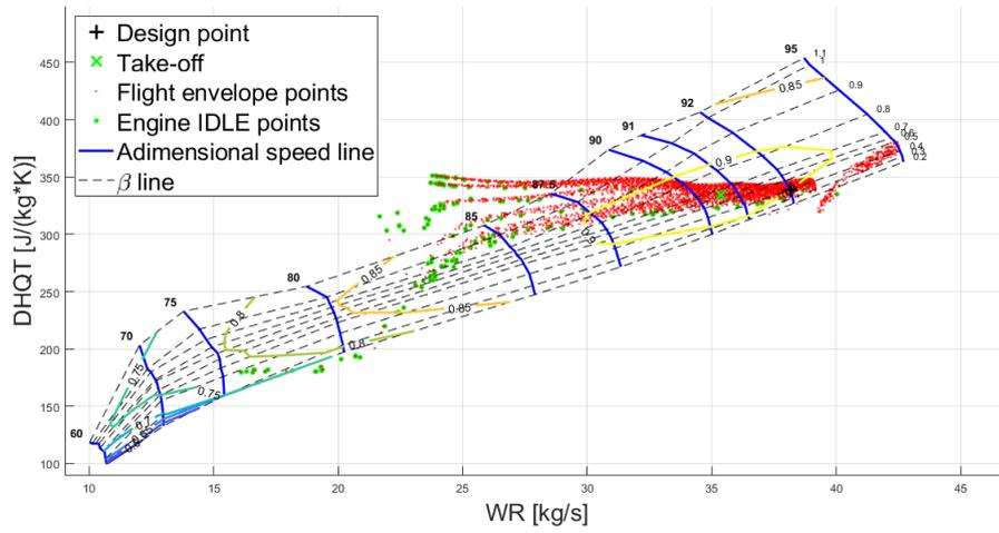
Figure 4.6: CFM56-7B24 LP compressor performance map.
