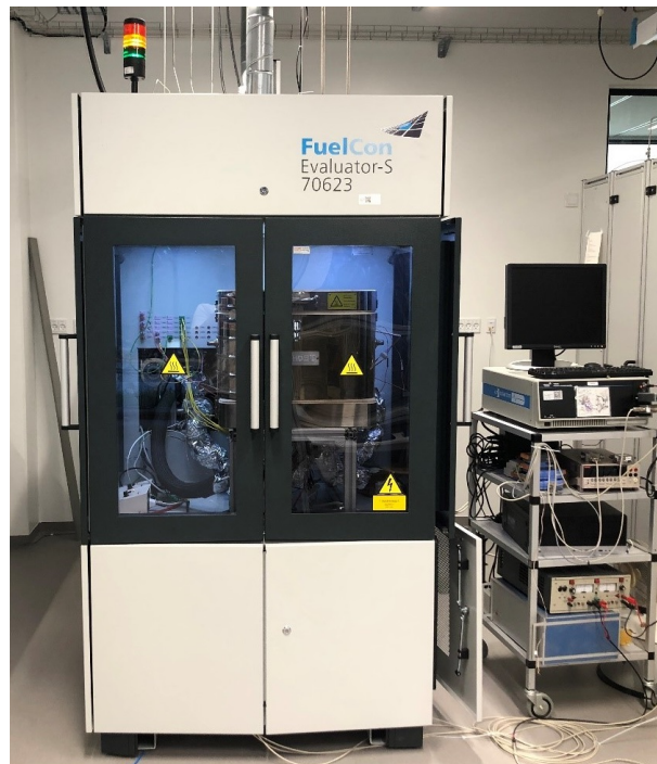
Figure 3.1: Stack testing station (Rig85).
