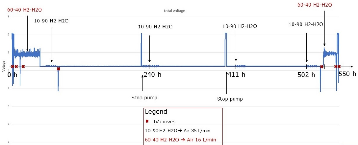
Figure 5.10: Voltage during 500 h for stack A.
