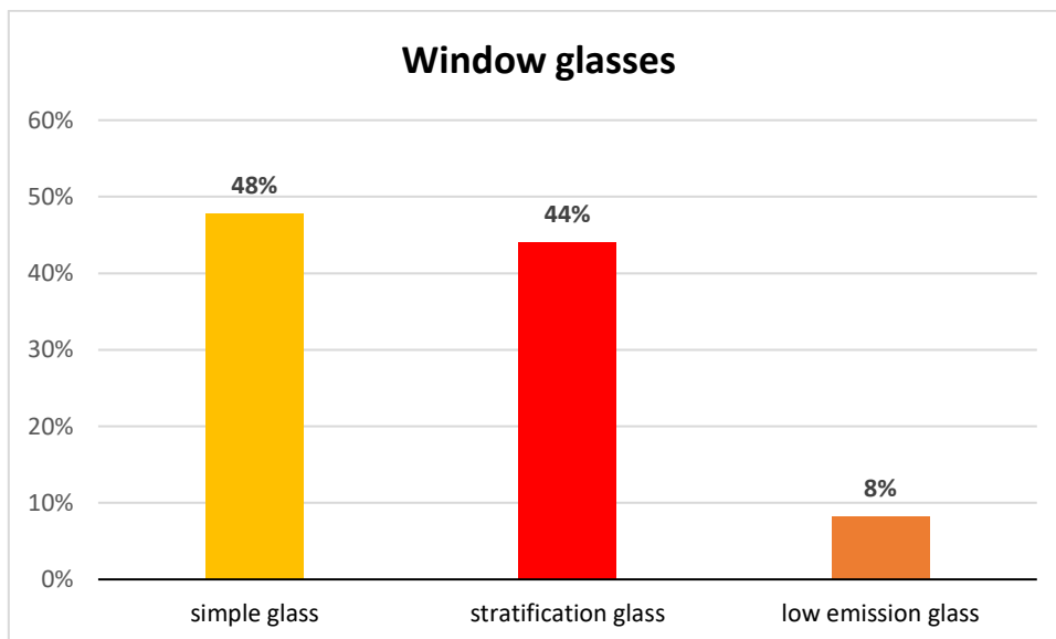
Figure 46: window glasses in school buildings under the direct administration of the Municipality of Milan
