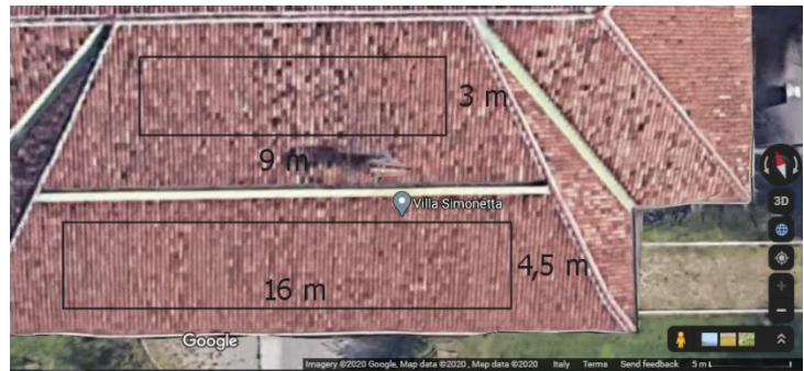
Figure 72: Total surface available for the installation of PV flat in the South-West facing rooftops according to an analysis conducted using through Google Maps
