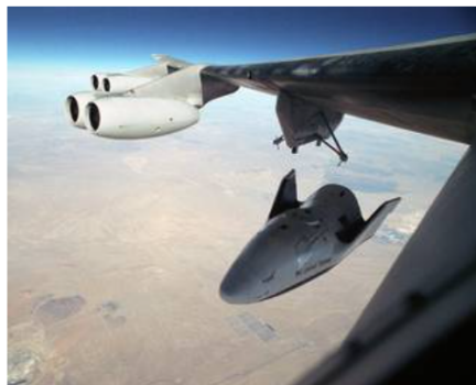
Figure 27: The X-38 prototype of the Crew Return Vehicle for the International Space Station drops away from its launch pylon on the wing of NASA's NB-52B mothership as it begins its eighth free flight on Thursday, Dec. 13, 2001. [NASA] [28]
