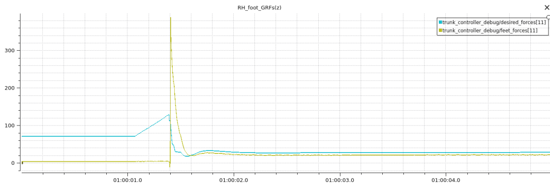
(c) Desired GRF on the RH foot on the z axis (in blue) and the actual reaction force
