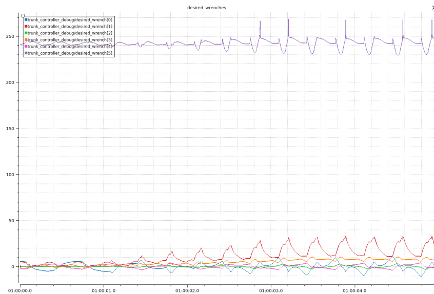
Figure 5.6: Desired wrenches of the Aliengo robot. The z axis wrench (in purple) is clearly the main component but, when the robot starts climbing the plane (at around 1:00:02) a much higher component on the rotational y axis (in red) can be appreciated
