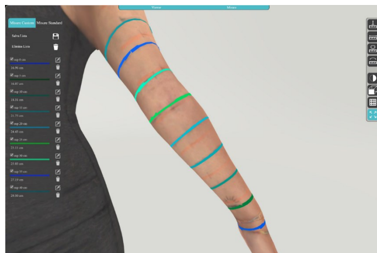
Figure 43 - Circumferential measurements taken with a virtual tape, in this case according to the fixed-heights technique.
