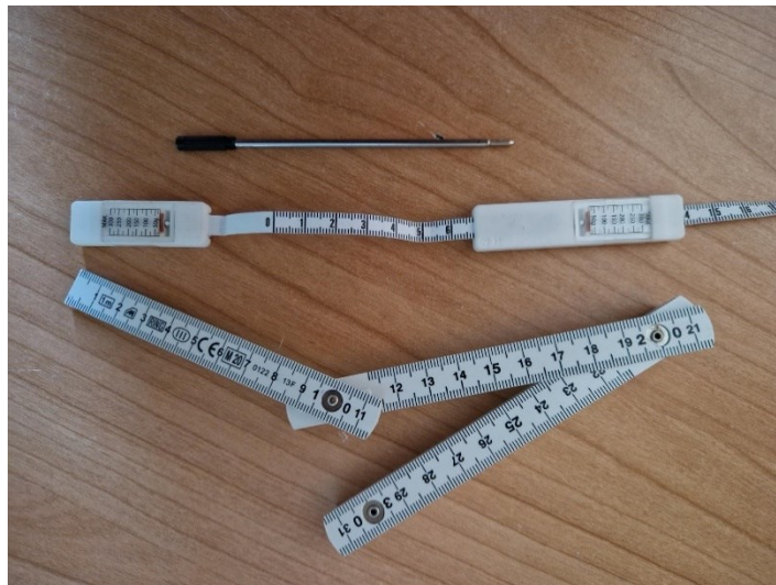
Figure 7 - Instruments for centimetric measurements: thin pen (top), tape measure with sliding dynamometer (middle), rigid folding plastic tape (bottom)
