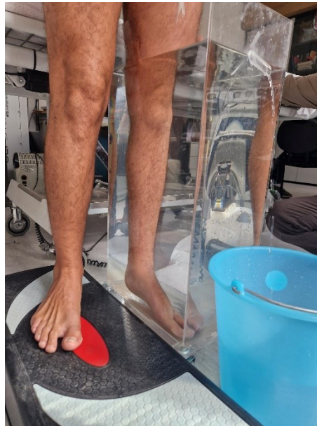
Figure 24 - Patient standing on the adjustable platform with the oedematous limb submerged in water up to the point E1.
