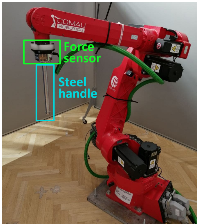
Figure 5.2: The Comau Smart Six manipulator equipped with the F/T sensor and the steel handle.
