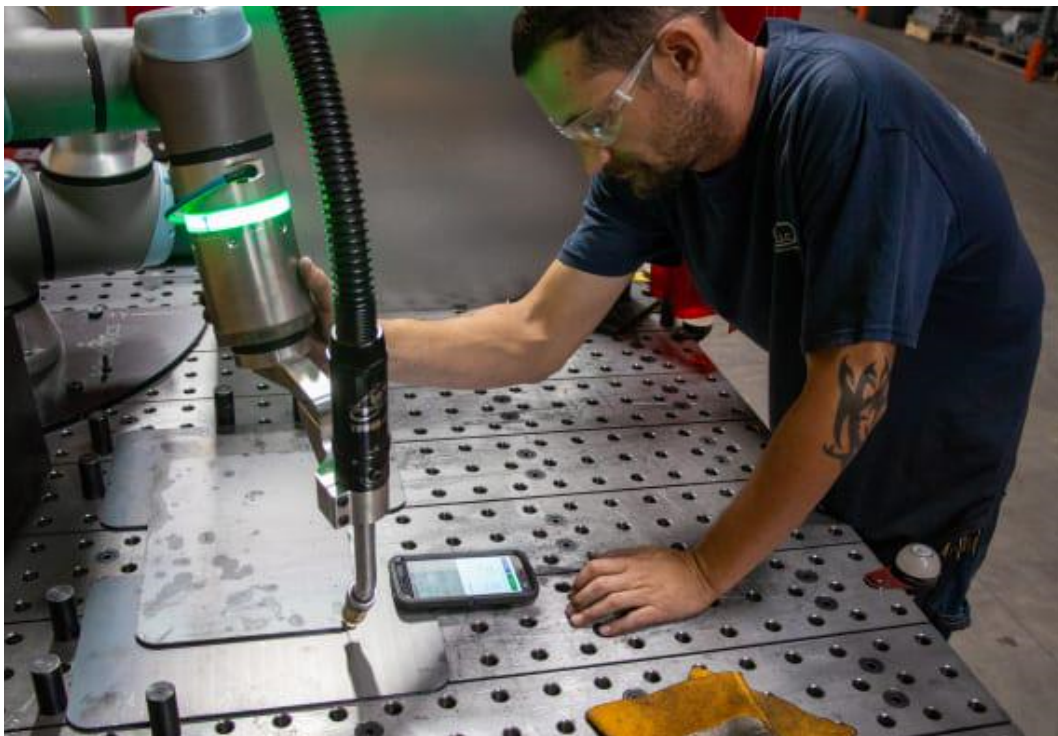
Figure 1.3: Example of a collaborative welding operation.
