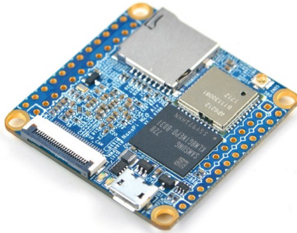
Figure 6.51: NanoPi NEO Air companion (source [2])
