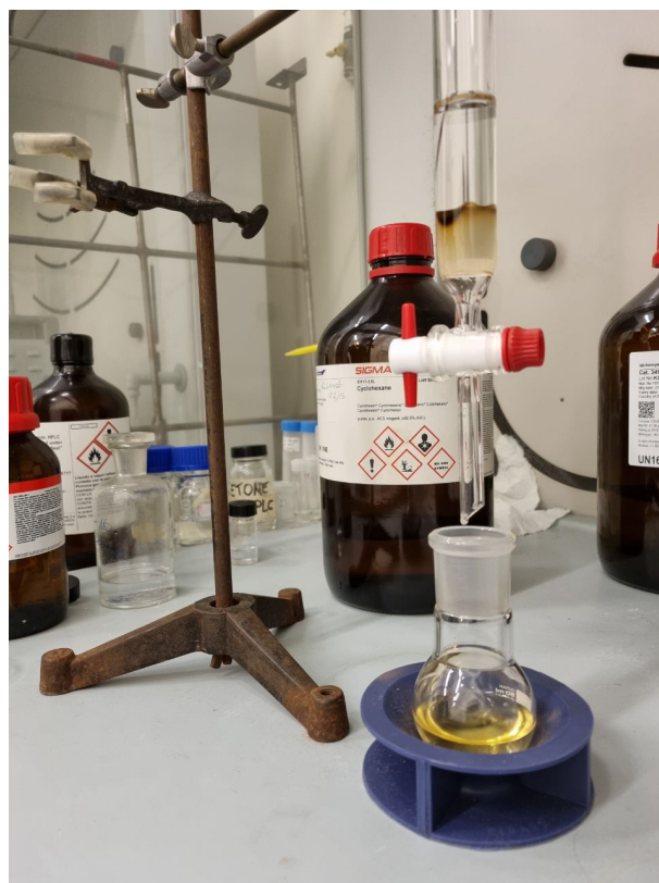
Figure 3.5: Collection of the purified eluate through the silica-gel column.
