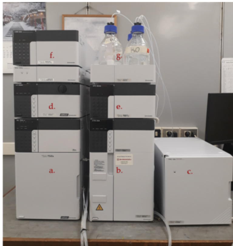
Figure 3.6: HPLC setup: a) autosampler; b) oven and columns; c) fraction collector; d) quadripartite pump system; e) photodiode array spectrophotometer; f) controller; g) solvent tray [101].
