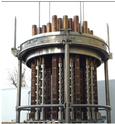
Figure 5.1: Top of a control cluster
