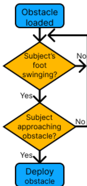
Figure 2, flow diagram of the control system for the tripping setup.
