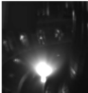
Figure 5.5: IR camera snapshot documenting material detachment from the DiMES sample. Images courtesy of C. Lasnier and I. Bykov.
