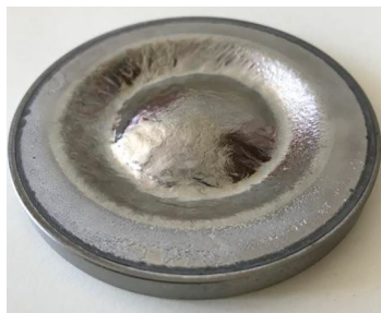
Figure 3.3. Photograph of a titanium target after use. The racetrack is perfectly visible.
