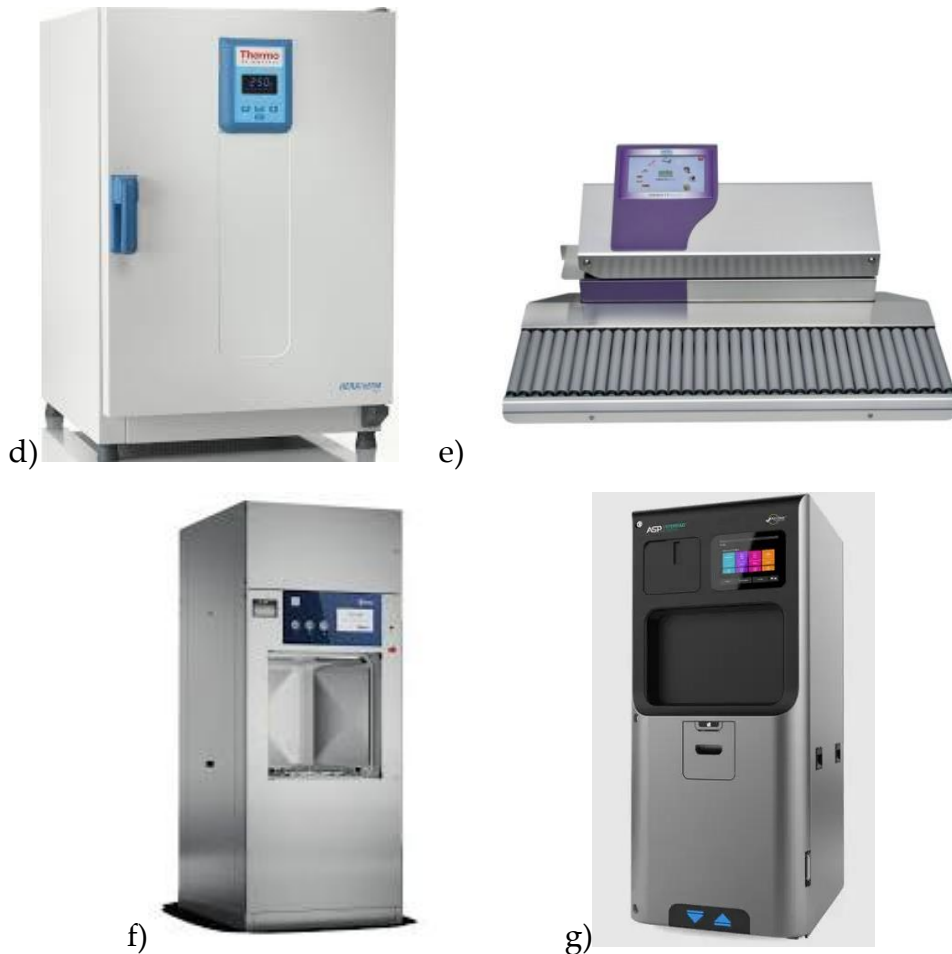
Fig. 8: CSSD 2's equipment: a) DS 1000 2S washer disinfecter; b) LC 20/2 containers washer disinfecter; c) LC 80/3 cart washer disinfecter; d) Heratherm OMS 180 instrument Drying Cabinet; e) MINIRO' H-LAN TOUCH heat sealers; f) VS 8/2 E Steam Sterilizer; g) STERRAD 100 NX Sterilizer
