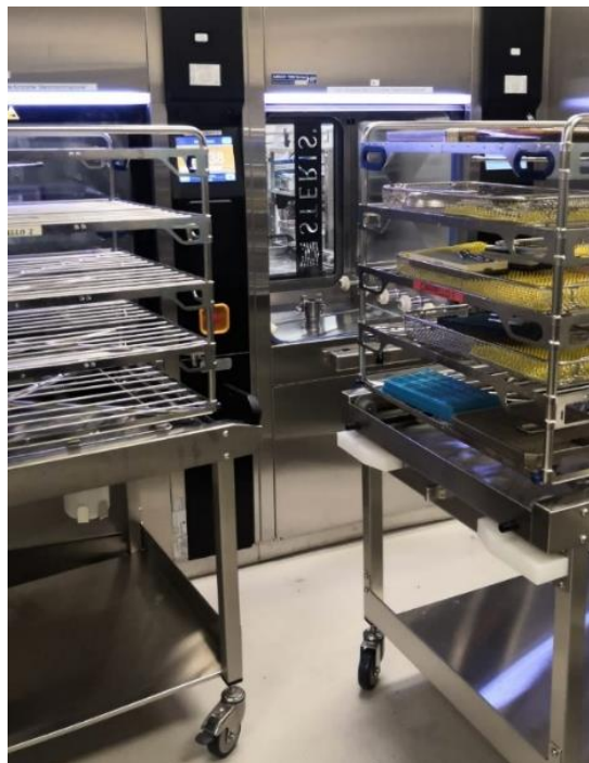
Fig. 14: loading of the washer disinfector at the beginning of the washing phase
