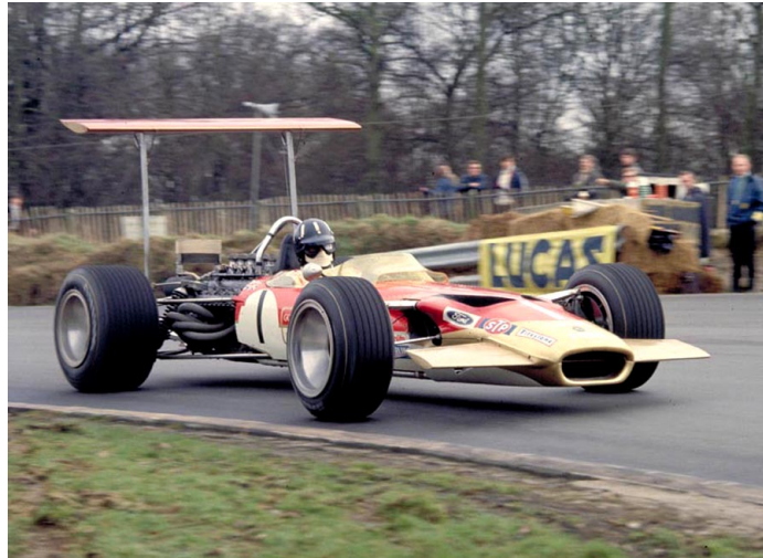
Figure 1.1: First appearance of front and rear wing on the Lotus 49 in 1968 [1].
