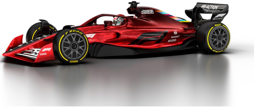
Figure 1.2: Formula 1 2022 prototype. The bodywork is cleaner and simpler. Despite the current cars, not so many aerodynamic devices are present as suggested by FIA new regulations, simplifying the body and the flow around the car.
