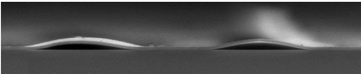
Figure 4.2 Example of detachment of the film present in the annealed samples deposited at room temperature.
