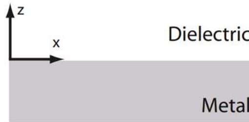
Figure 1.5 Schematic representation of the geometry of propagation of SPPs along the interface [1].
