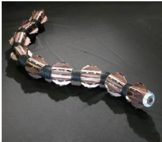
Figure 2.6: ACM-R5 amphibious snake robot, developed by Hirose et al.
