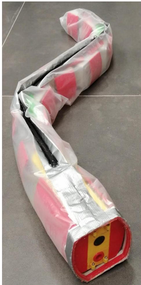
Figure 6.11: The assembled ASR with the waterproofing polythene cover.
