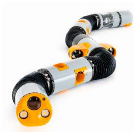
Figure 2.12: Snake robot with active propellers
