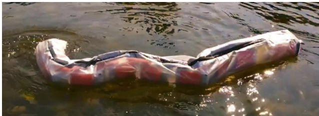
Figure 6.13: Aquatic snake robot performing the eel-like motion.
