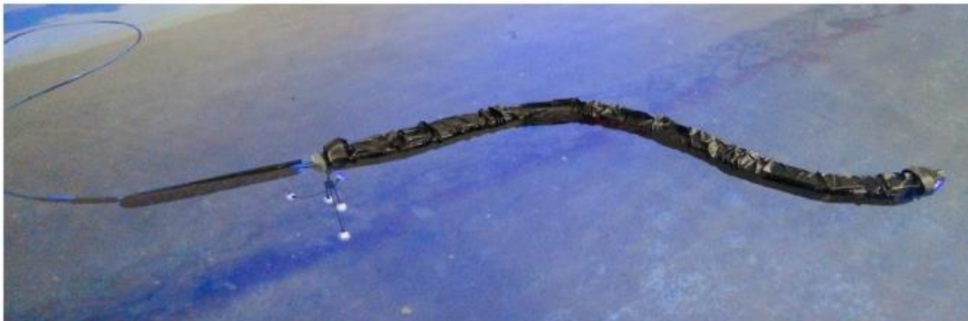
Figure 2.7: Mamba snake robot with passive propellers.
