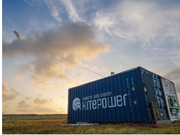
Figure 1.4: Kitepower Falcon (see [11]), a soft kite with ground level generation and its ground station/container (6.06m length x 2.44m width x 2.60m height), with an overall weight of 9.5 tons)
