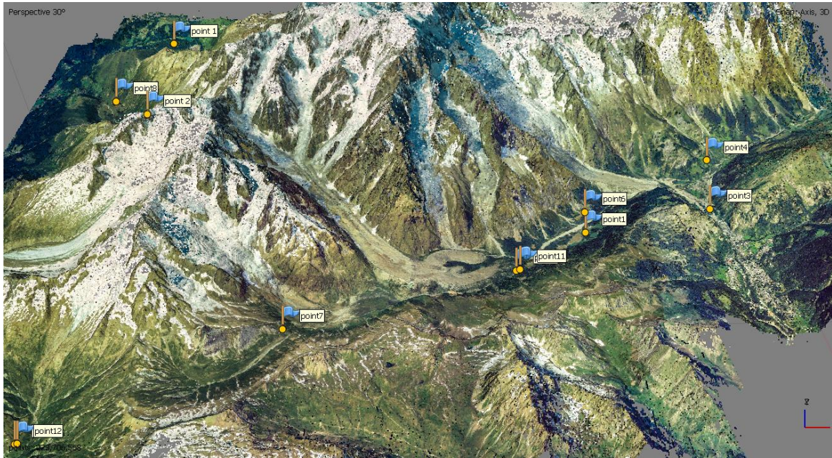
Figure 3.10. Area of interest in 3D dense cloud from 2001 dataset, Location and distribution of GCP's for dataset 2001.
