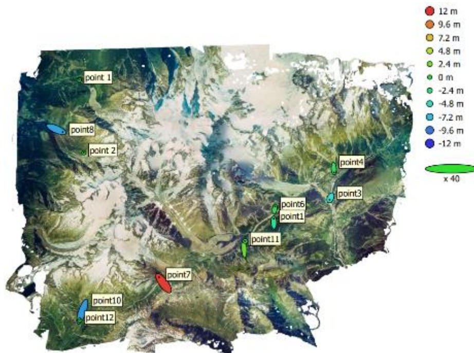
Figure 3.4. Example position and distribution of GCP's over the Val Veny mountains in one of the datasets
