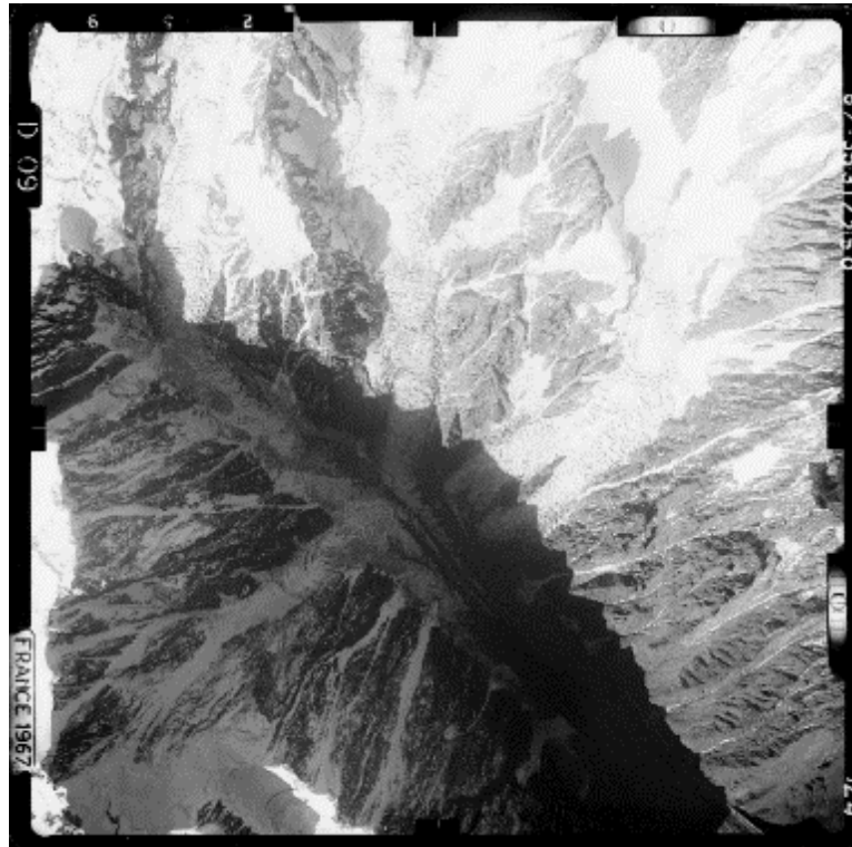
Figure 3.22. Effect of shadows on the upper parts of Miage glacier that avoid proper point extraction and 3D reconstruction in dataset of 1967.
