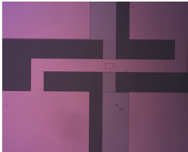
Figure 4.20: Zoom on the pillar region of the optical microscope image of the device. The dark edges of the pillar represent the photoresist leftover.
