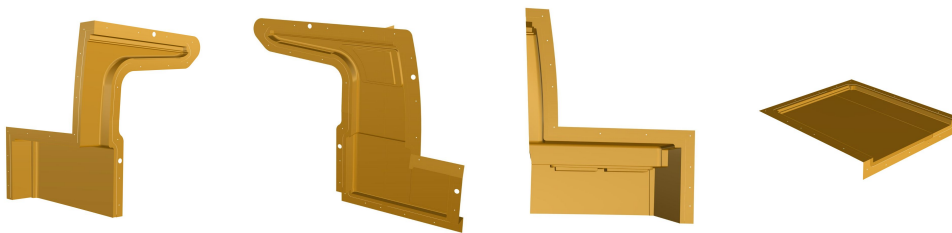
Figure 3.12: Starboard side T-Top leg moulds decomposition.
