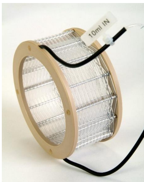
Figure 4 - 10 mL standard coiled tubular reactor
