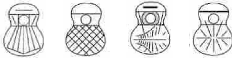
Figure 2.2: Different bracing systems for classical guitars. From left to right: Torres, lattice, Kasha and radial.
