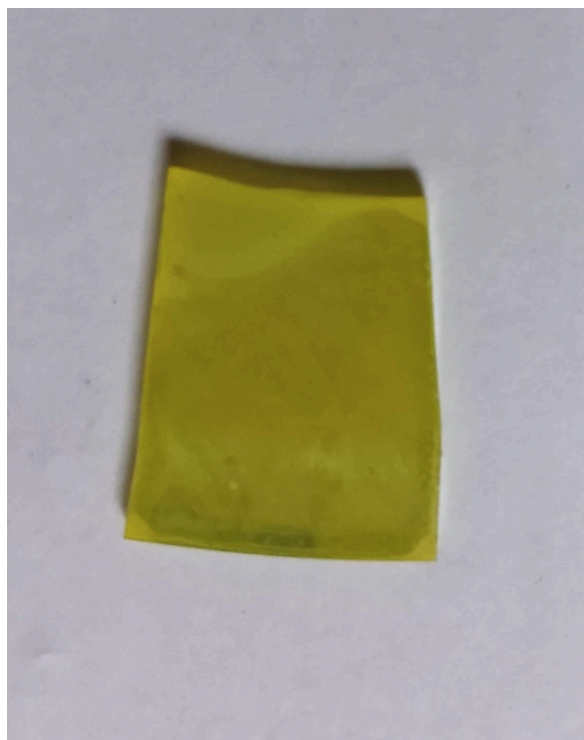
Figure 51. Evaporation defects present on the surface of a photoanode prepared via drop casting of 10 \mu\text{L}/\text{cm}^2 of \text{Mo}:\text{BiVO}_4 solution over a \text{BiVO}_4 seed layer.
