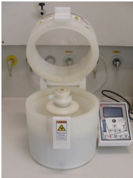
Figure 29. Picture of the spin coater employed for this work. A vacuum pump was also linked to it through a plastic pipe, in order to keep samples in position during rotation.
