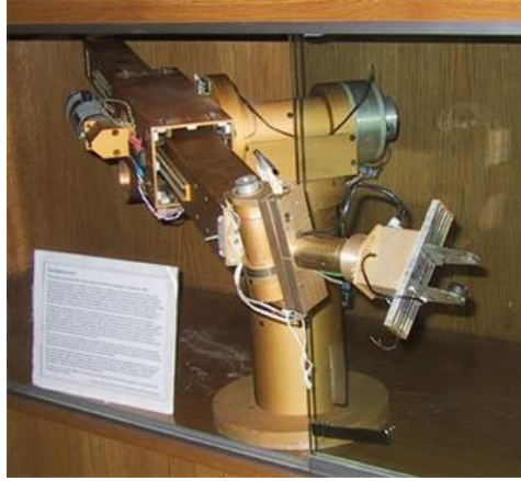
Figure 1.2: Example of robot of second generation (The Stanford Arm).
