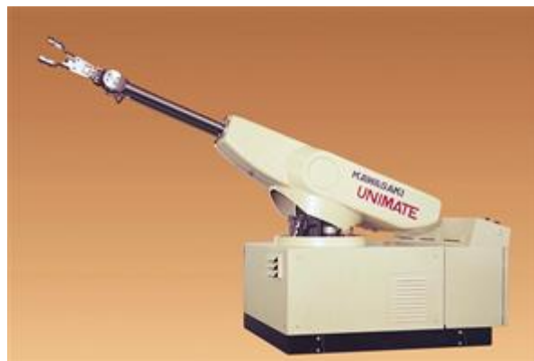
Figure 1.1: Example of robot of first generation (the Unimate robot).
