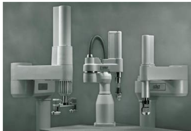
Figure 1.3: Example of robots of the third generation (AdeptOne SCARA robots)
