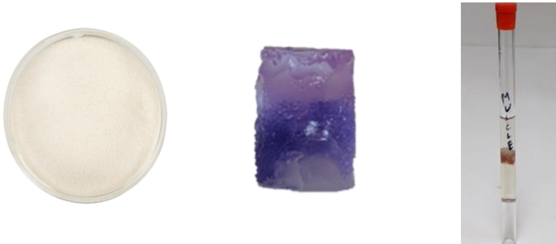
Figure 2.2: The examined sample. From left to right: gelatin sample, anisotropic phantom, mouse muscle sample
