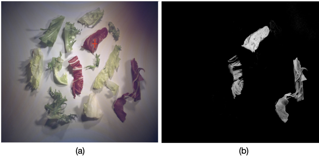
Figure 3.7: (a) RGB reconstruction of the samples and reference pixel. (b) Clustering for a spectral angle threshold \theta < 0.2 .
