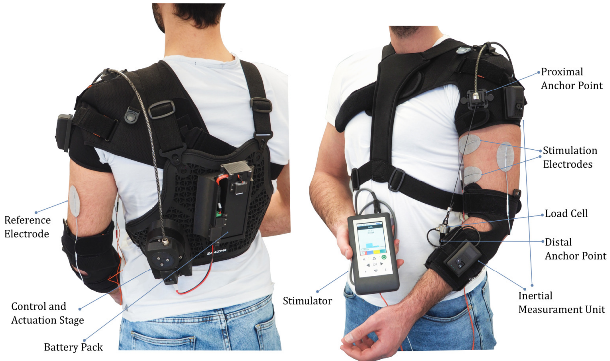
Figure 2.1: FES-exosuit Hybrid System for elbow flexion and extension: back view on the left and front view on the right.
