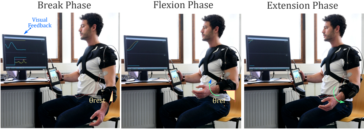
Figure 2.13: Phases of the State Machine . Example of one subject using the hybrid device. The Break, Flexion and Extension phases are shown. On the monitor of the computer the EMG signal and the two thresholds are shown to the subject in order to give to him a visual feedback regarding the extent of muscle contraction necessary to get to a threshold.
