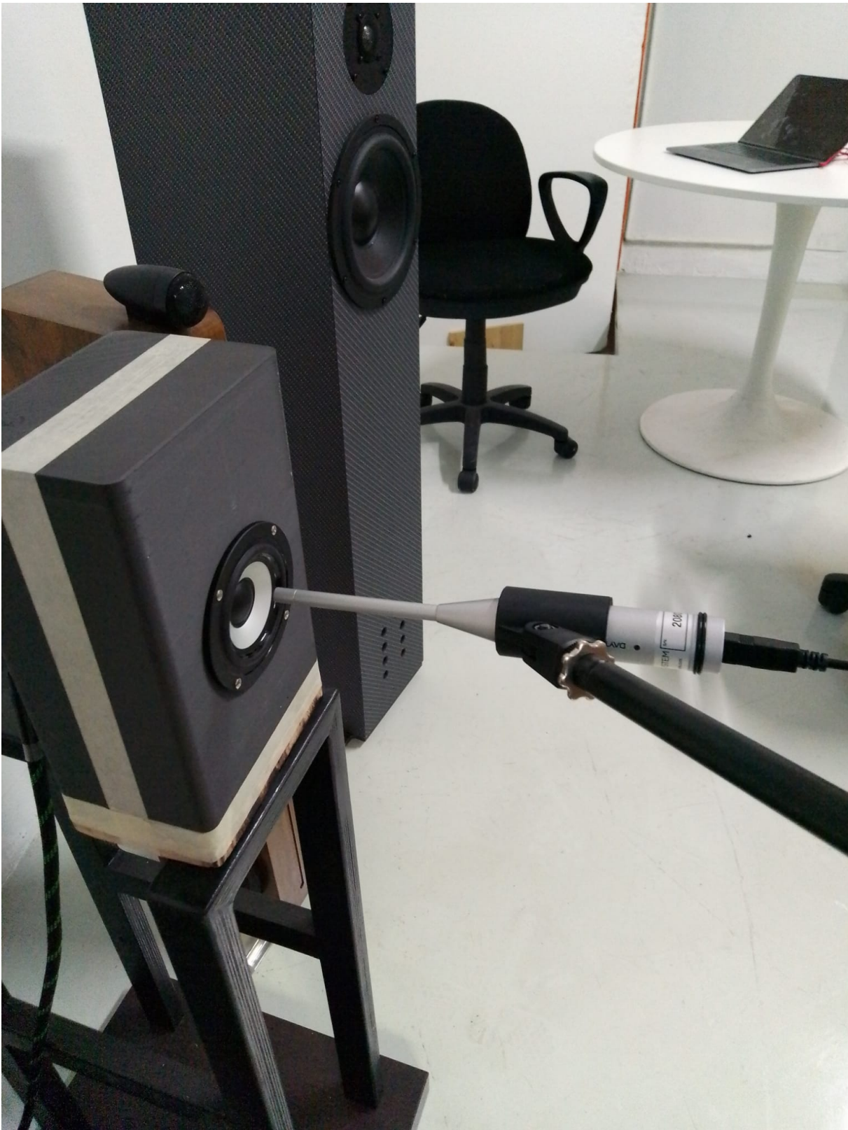
Figure 4.3: Near-field Recording of a R2c loudspeaker box
