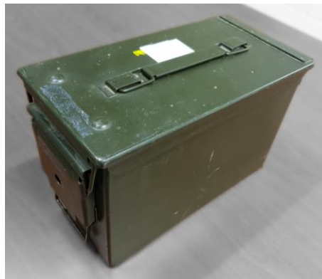
Figure 5.9 – Picture of the heavy box used as weight for the drop test. 16 kg (35.2 lb.).
