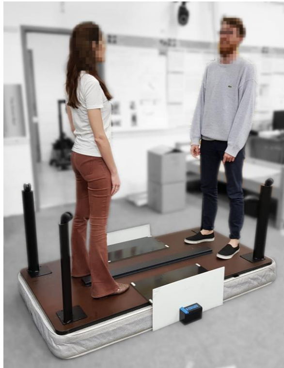
Figure 5.2 – Compression test of the mattress by means of a rigid wooden board (a table) and weights on it (two subjects, in this case).
