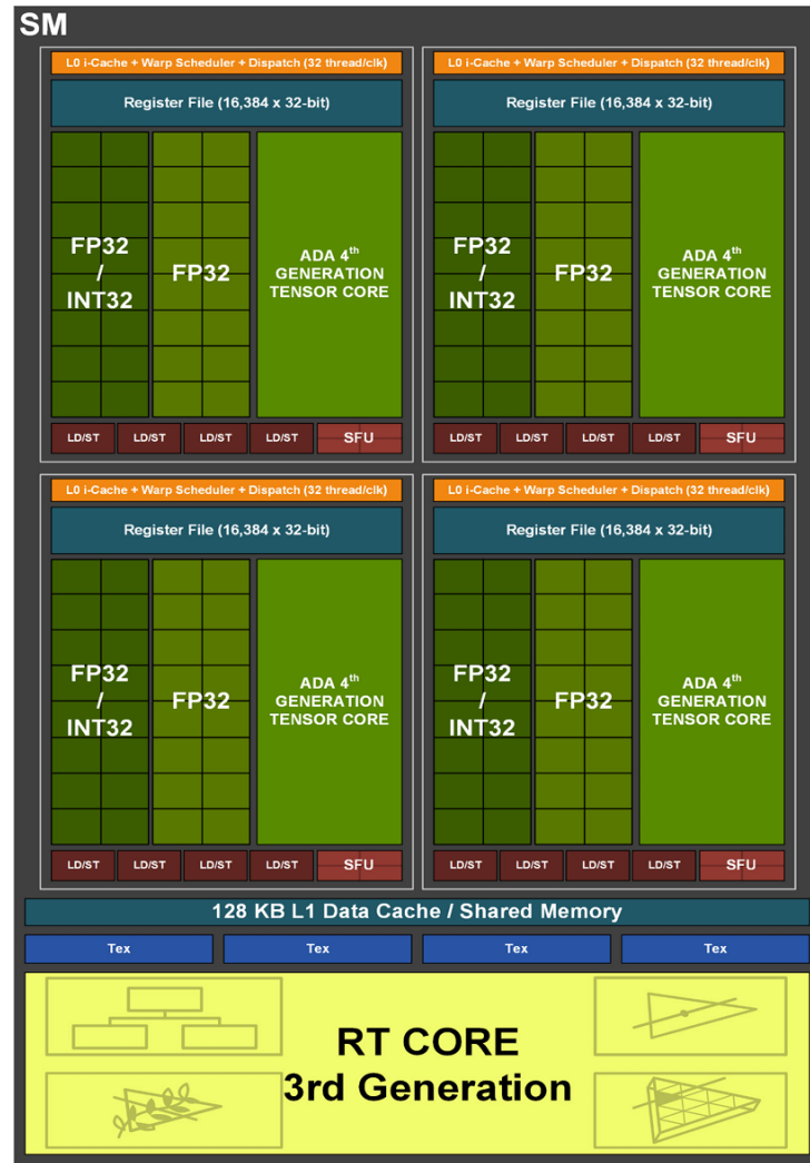
Figure 2.2: Internal architecture of a Streaming Multiprocessor (SM) in the NVIDIA Ada Lovelace architecture, showing the four Processing Blocks, the shared L1 cache and Texture Units [9].
