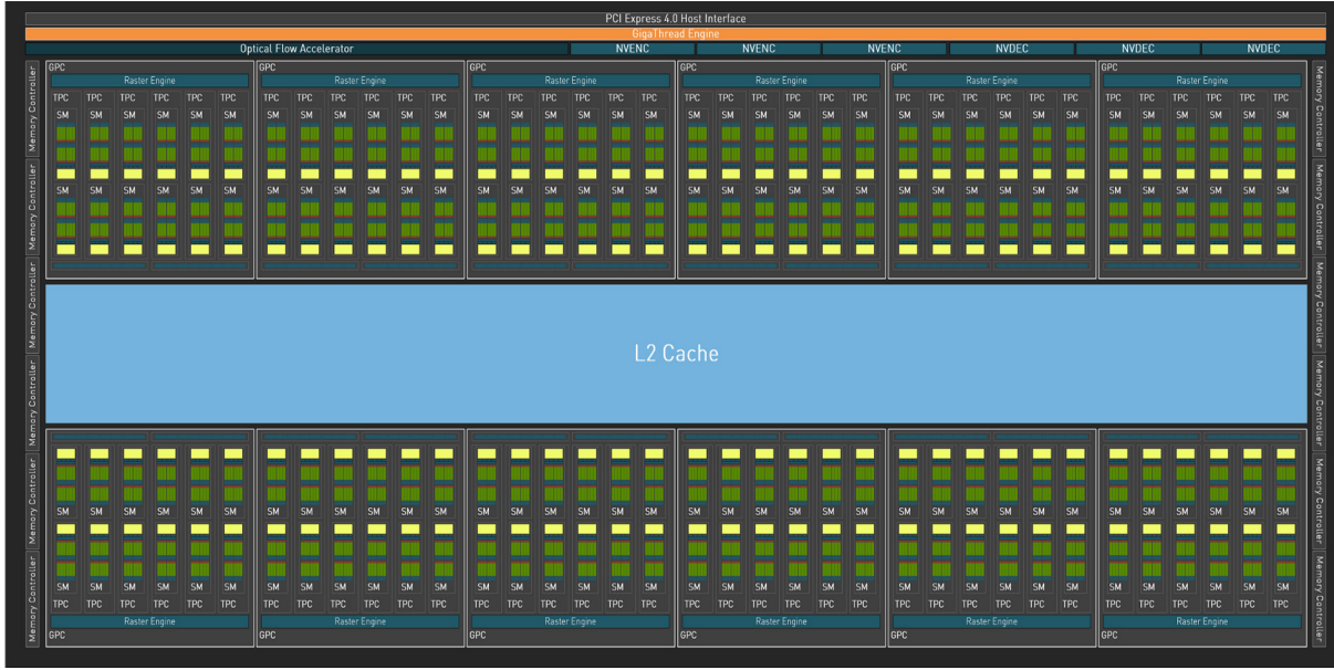
Figure 2.1: High-level architecture of an NVIDIA Ada Lovelace GPU, showing the hierarchy of GPCs, TPCs, and SMs sharing a common L2 cache [9].
