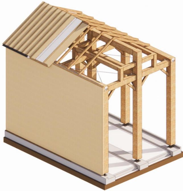
Figure 3-22 Primary and Secondary Structure Overlook (self-drawn by the author)
