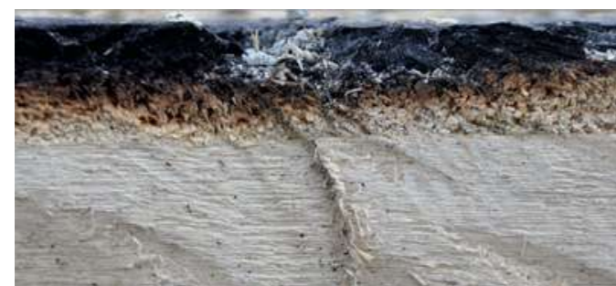
Figure 7.8 Fire resistance of CLT/ Outside layers of the sample are burnt while the inner core is still efficient from the structural point of view
