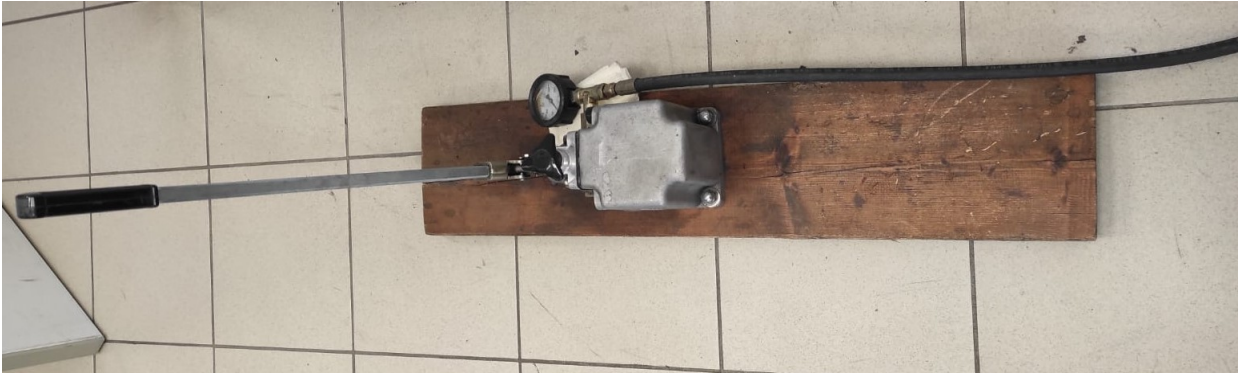
Figure 3.1: Hydraulic pump used for pressing the tablets.
