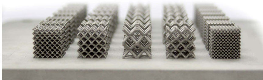
Figure 7 Lattice structures obtained with AM technology [90]
