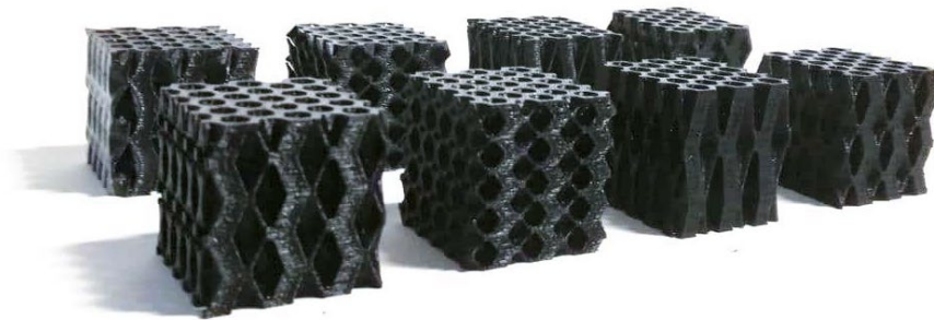
Figure 43 3D printed bio-inspired lattice structures
