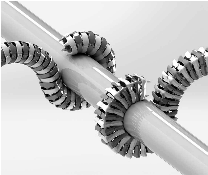
Figure 22 A round-plated tail, typical of seahorses (right): the square segments create more contact points with the surface that it is gripping. Image via Michael Porter/Clemson University.
