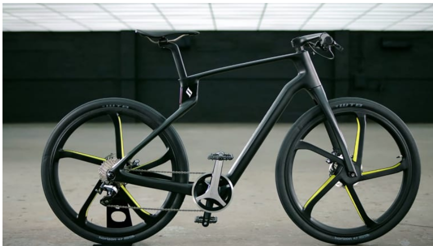
Figure 121 Carbon fibre 3d printed bike frame [104]
