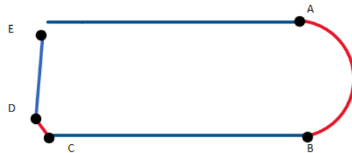
Figure 1: MoveL segments are depicted in blue, and complementary segments are depicted in red
