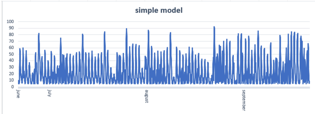
Figure 84: percentage of dissatisfied people for the summer in the simple model without shading
