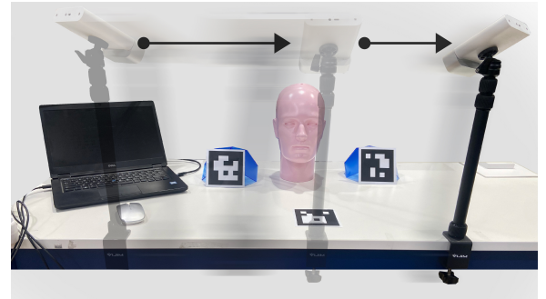
Figure 4: Proposed setup for the acquisition of multiple frames of the head phantom.
