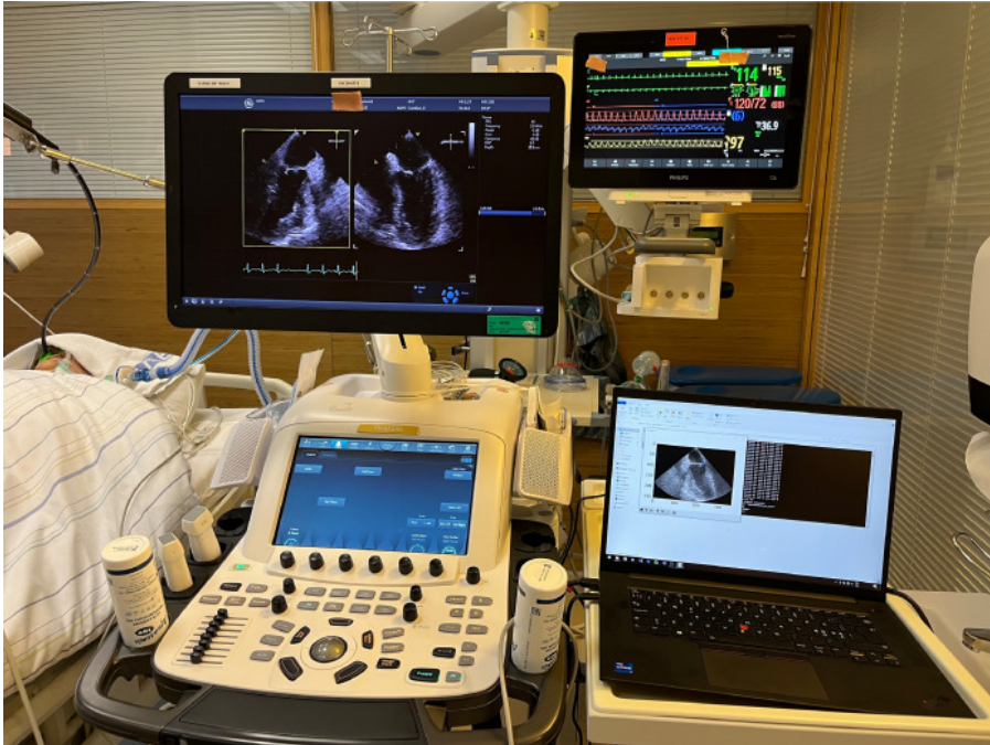
Figure 7: Application of Echocoder 2D+t in the ICU. A laptop provides the MAPSE measurement, together with visualizations, videos and plots. Taken from [64].
