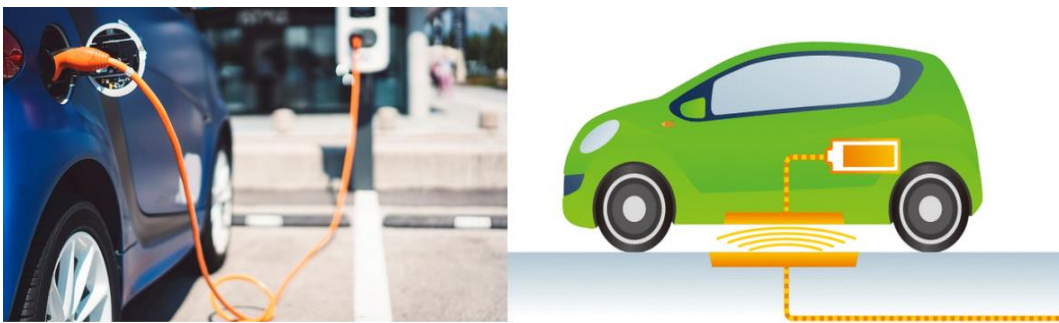
Figure 1-1: Charging System for EVs. Conductive Charging (a), Wireless Charging (b).
